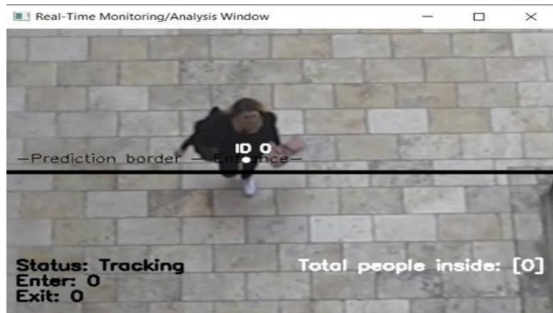
Figure 4: Tracking the movement of the person as he moves in and out
