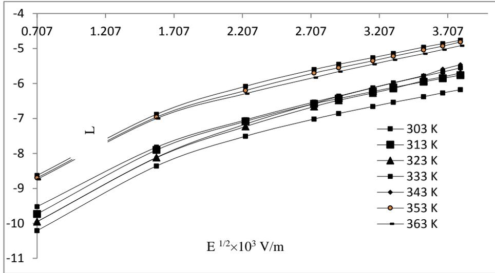
**Figure -1.** Plot of  $\ln J$  versus  $E^{1/2}$  for unpolarized sample.
