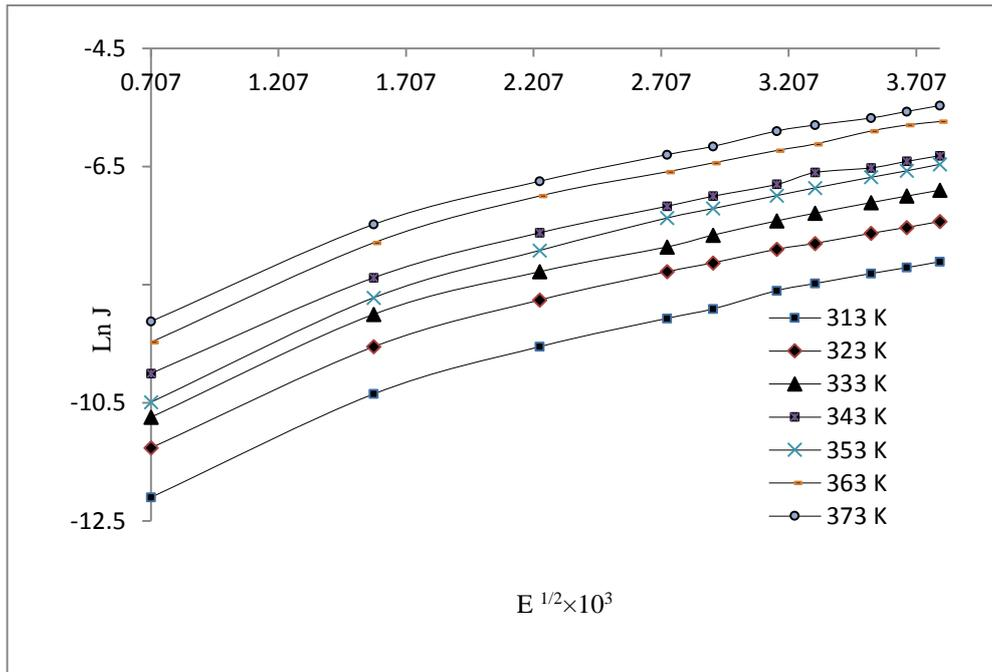
**Figure -2.** Plot of  $\ln J$  versus  $E^{1/2}$  for polarized sample.
