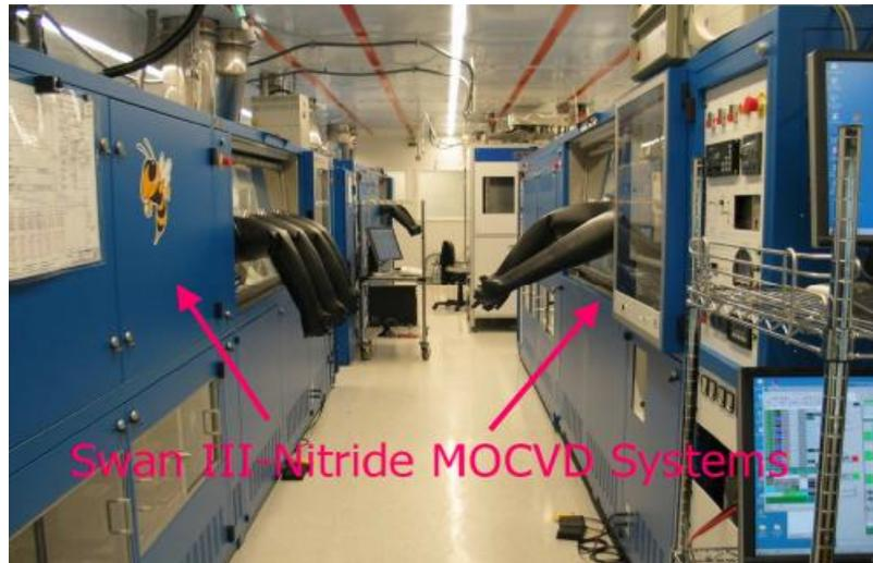
**Figure 3:** MOCVD III-N Systems. Two Thomas Swan CCS 6x2 MOCVD reactors used for the development of GaN/AlGaN based UV-APDs at Georgia Institute of Technology.
