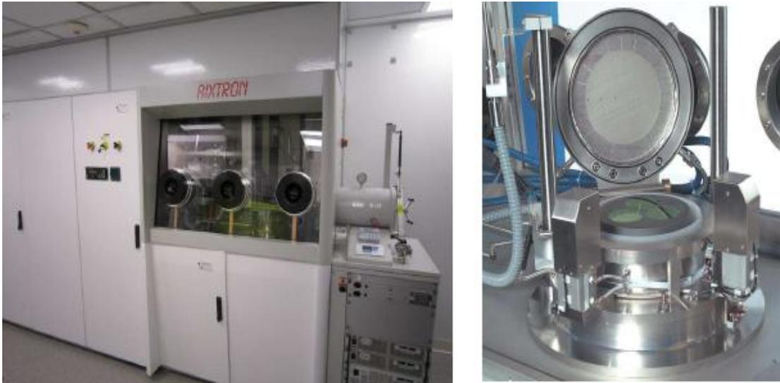
**Figure 4:** New-generation AIXTRON CCS 3x2"; High-temperature III-Nitride 3x2" MOCVD growth chamber open for loading wafers and showing close-coupled showerhead.
