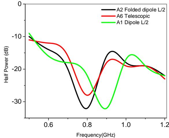
**Figure: 3 Shows beam width variation for different antennas.**
