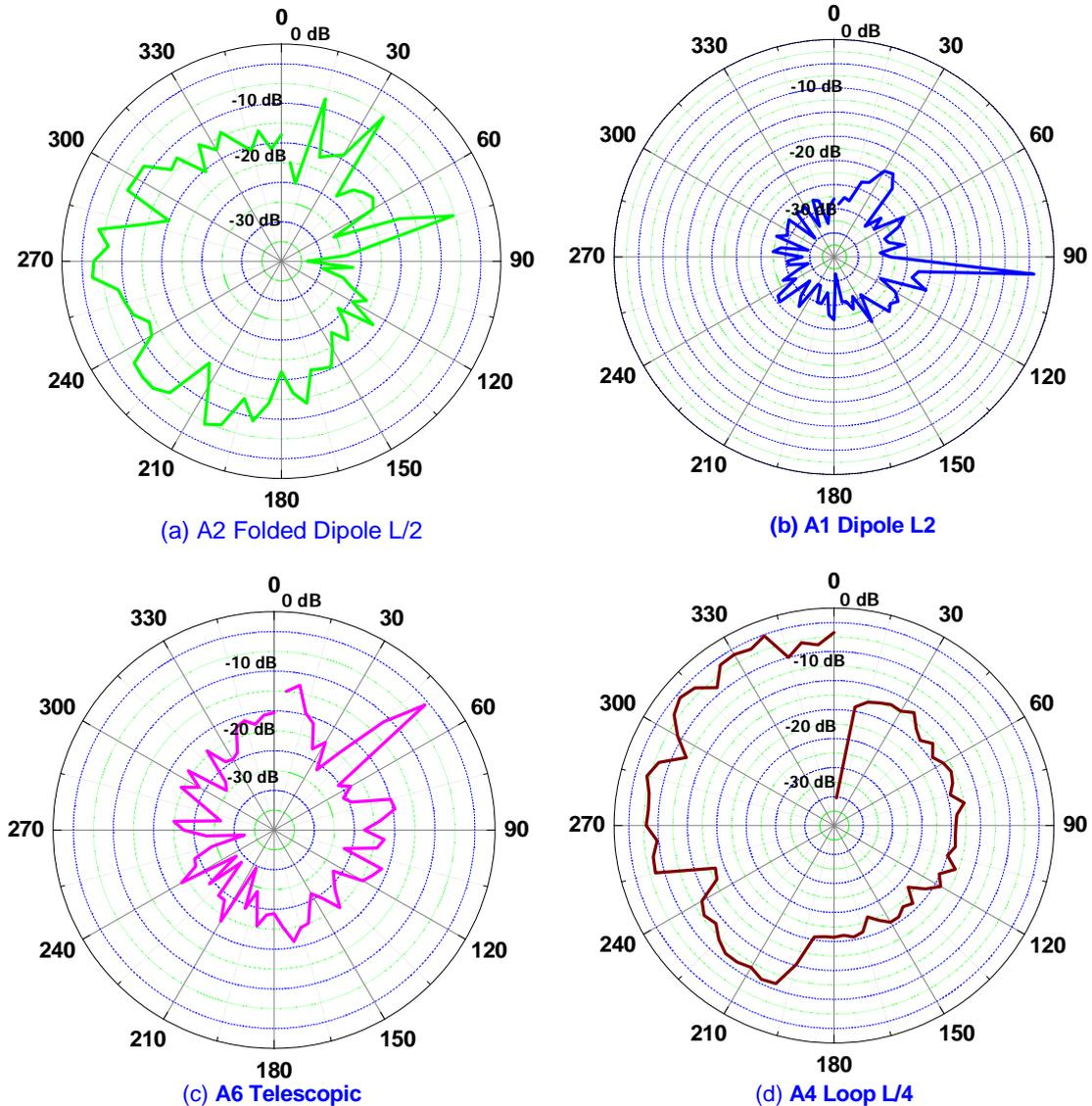
**Figure: 2 Shows radiation pattern of (a) A2 folded dipole L/2 (b)A1 dipole L2 (c) A6 Telescopic (d) A4 Loop L/4.**
