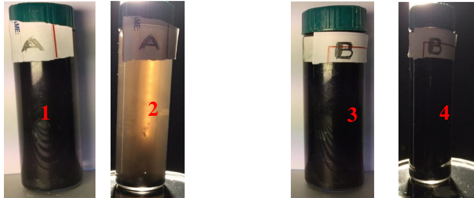
Figure 4a: Fluid A: Mechanically mixed (1) Right after mixing (2) After 24 hr.
