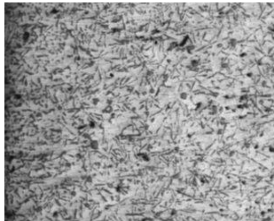
Fig. 8 Optical microstructure of matrix alloy (LM 13) at 200X
