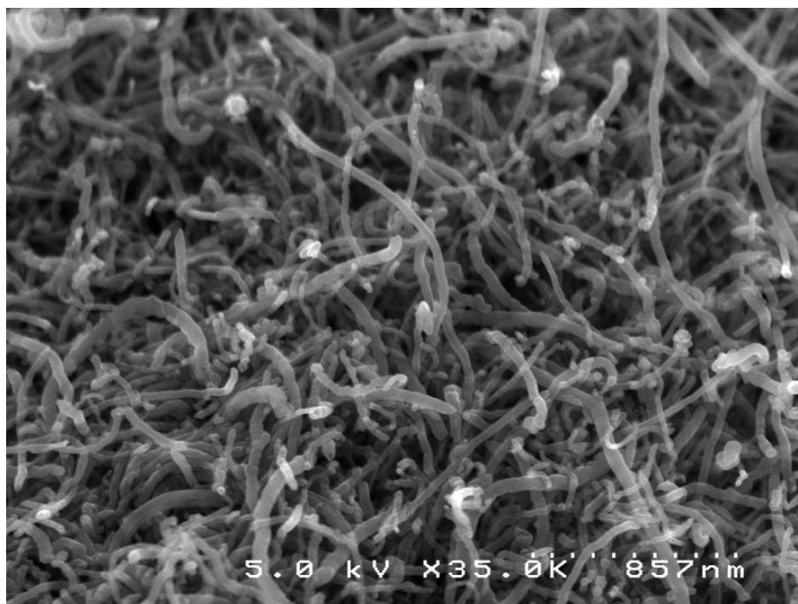
**Fig. 5.** SEM image of the MWCNT after five irradiation and cooling cycles.
