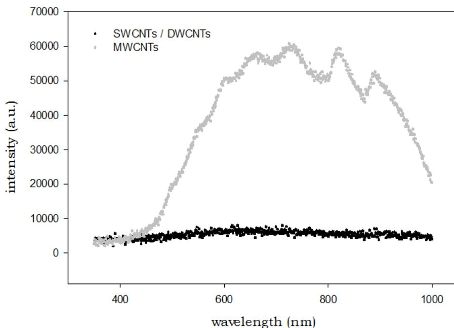
**Fig. 3.** Comparison of the sums of radiation spectra emitted by the > 90 wt% SWCNT/DWCNT and the > 95 wt% MWCNT (> 50 nm diameter) samples during three 25 s microwave irradiations.
