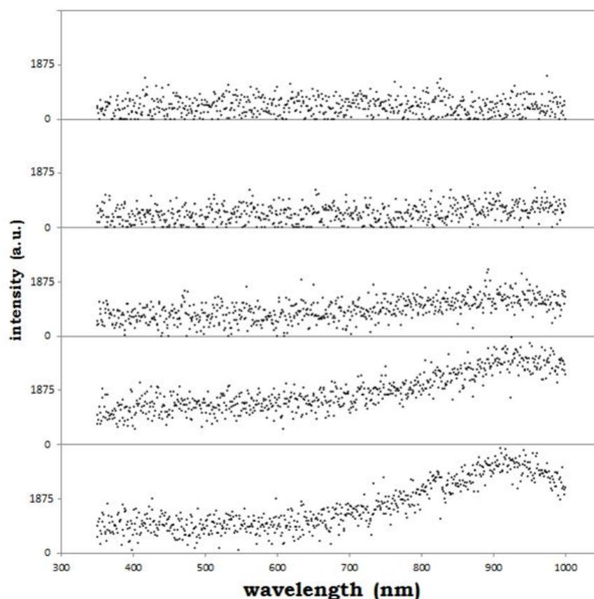
**Fig.1.** Spectra of radiation emitted by the SWCNTs/DWCNTs during several irradiation and cooling cycles (with background subtracted). From top to bottom, the spectra correspond to the first, second, third, fourth, and fifth cycles.
