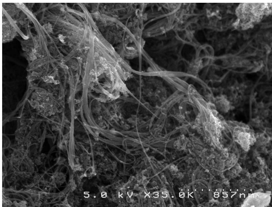
**Fig. 4.** SEM image of the SWCNT/DWCNT sample, as purchased.
