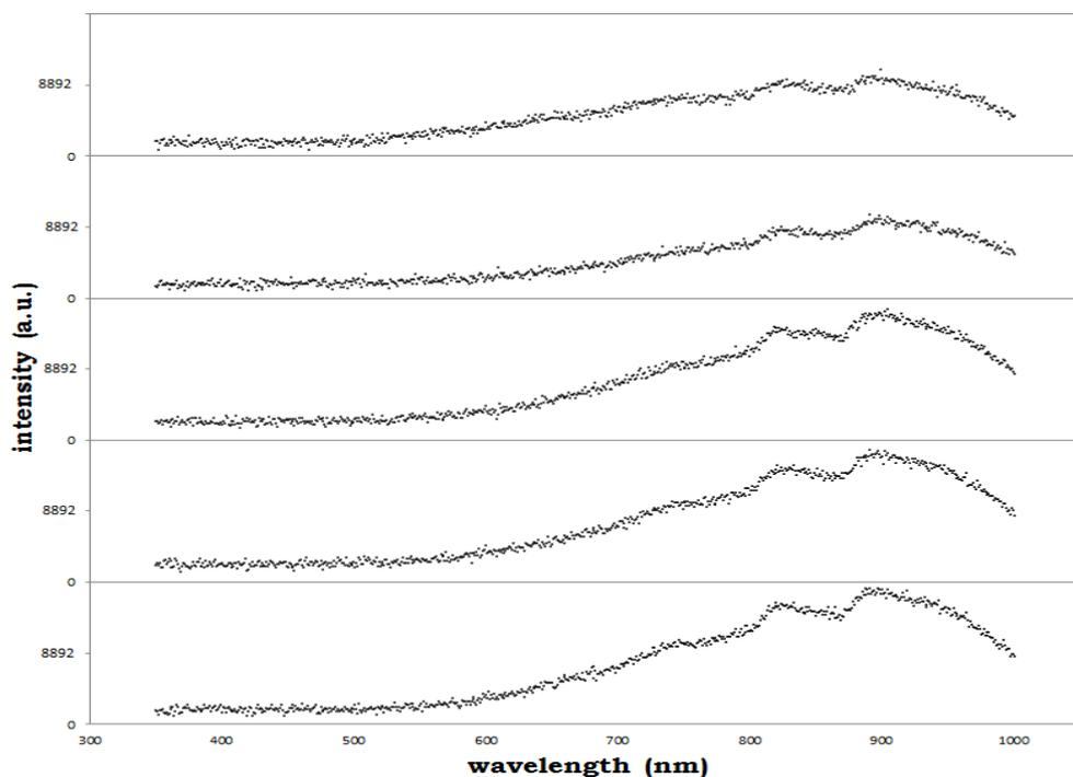
**Fig. 2.** Spectra of radiation emitted by the MWCNTs during several irradiation and cooling cycles (with background subtracted). From top to bottom, the spectra correspond to the first, second, third, fourth, and fifth cycles.
