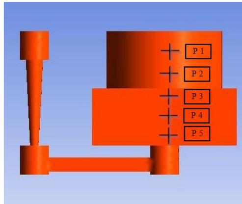
**Figure 4.** Location of 5 points in casting and riser
