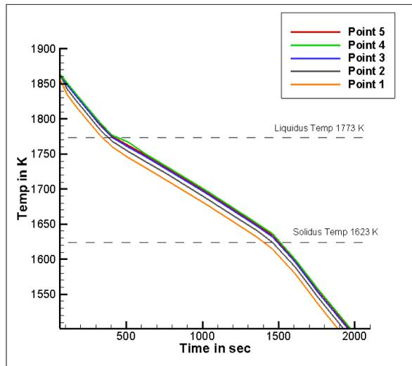
**Figure 8.** Temp Vs. Time graph case 2) 500 KJ/Kg
