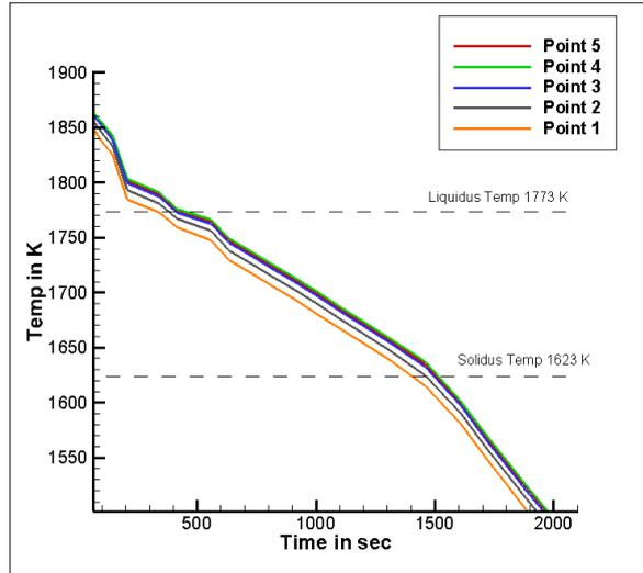
**Figure 7.** Temp Vs. Time graph case 1) 1000 KJ/Kg
