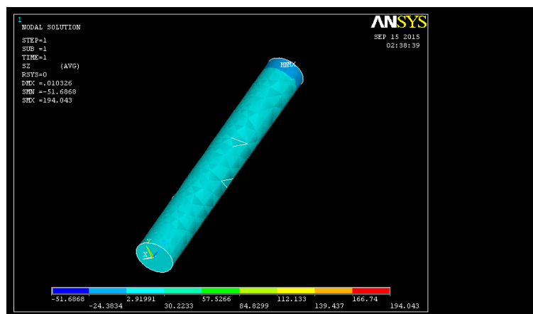
Fig.3 FEA results of UTS of hypereutectic Al-13 Si alloy.
