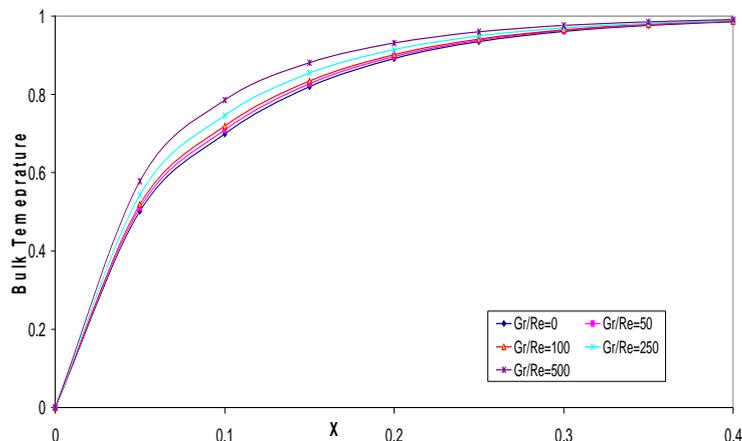
Fig. 9(c) : Bulk Temperature ( $\theta_b$ ) for fixed  $r_1=1$  and  $M=5$
