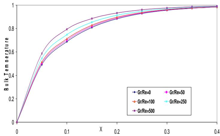
Fig. 9(a) : Bulk Temperature( $\theta_b$ ) for fixed  $r_1=1$  and  $M=0$
