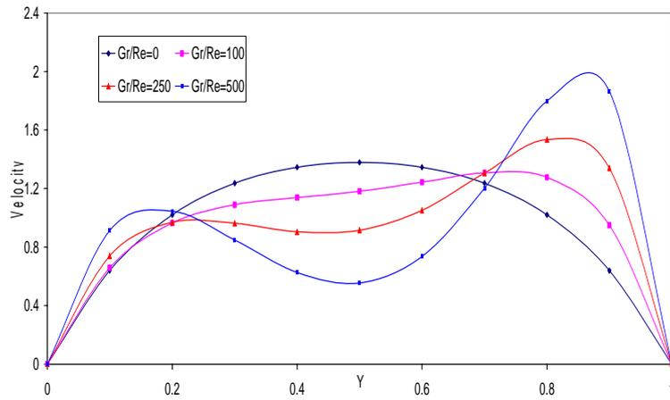
Fig. 4(c) : Velocity value for fixed  $rT=0.5$ ,  $X=0.04$  and  $M=5$
