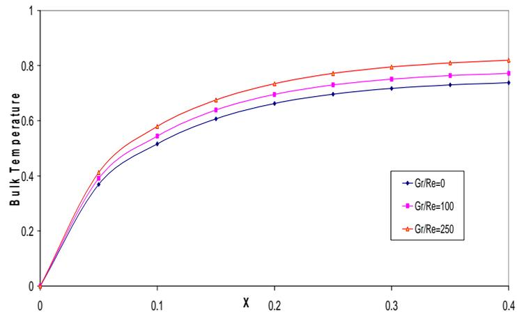
Fig. 8(a) : Bulk Temperature ( $\theta_b$ ) for fixed  $r_1=0.5$  and  $M=0$
