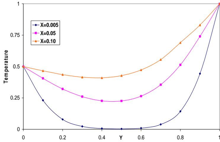
Fig.6(c): Dimensionless temperature distribution at  $r_1=0$ ,  $Gr/Re=250$  and  $M=5$
