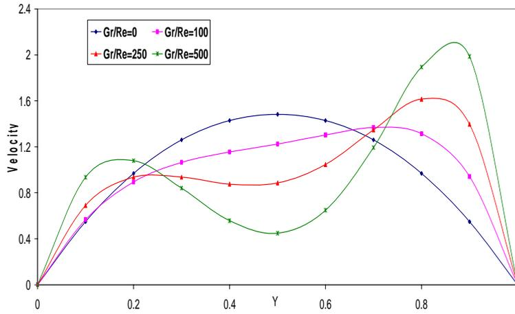
Fig. 4(a): Velocity value for fixed  $r_1=0.5$ ,  $X=0.04$  and  $M=0$
