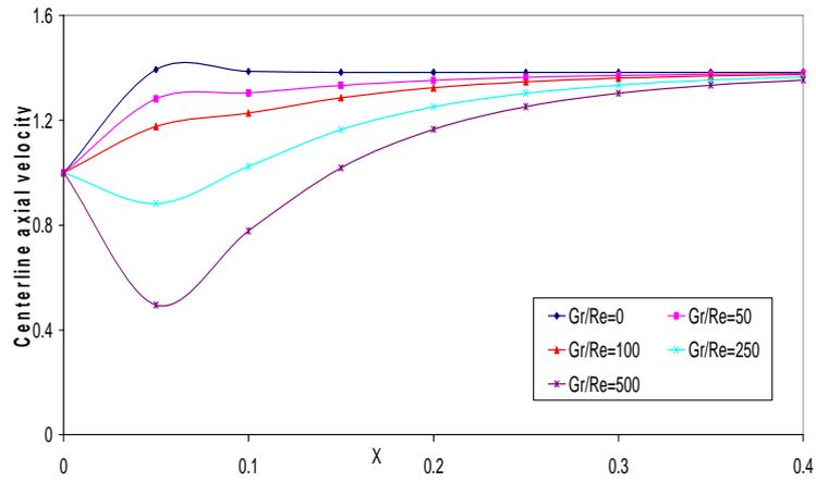
Fig.3(c): Centerline axial velocity values for fixed  $r_1=1$  and  $M=5$
