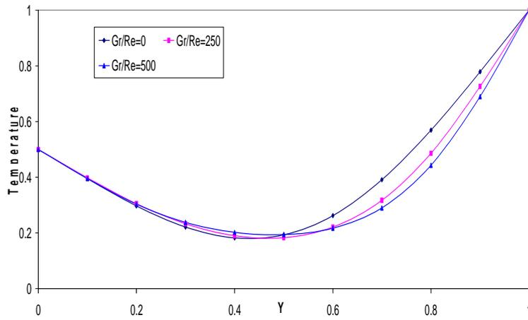
Fig.5(c): Temperature value for fixed  $r_1=0.5$ ,  $X=0.04$  and  $M=5$
