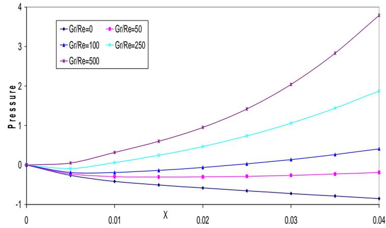
Fig.7(a): Pressure values for fixed  $r_1 = 1.0$  and  $M = 0$
