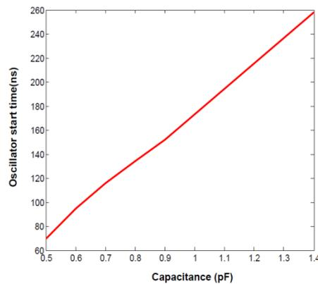
**Figure 6(b):** Oscillator start time vs Capacitance ( $I_{\text{bias}}=2\mu\text{A}$  constt)
