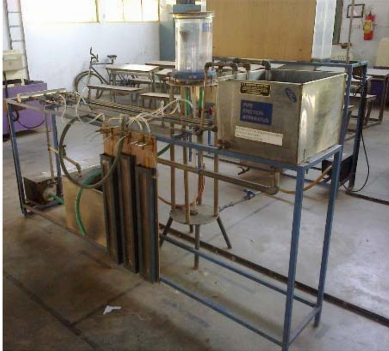
**Fig.2.1. Model of a Pipe Friction Apparatus**
