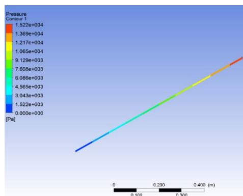
**Fig.2.3. Pressure counter diagram for water (liquid)**
