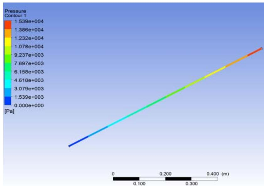
Fig.2.7. Pressure counter diagram for CuO + water (liquid) particles
