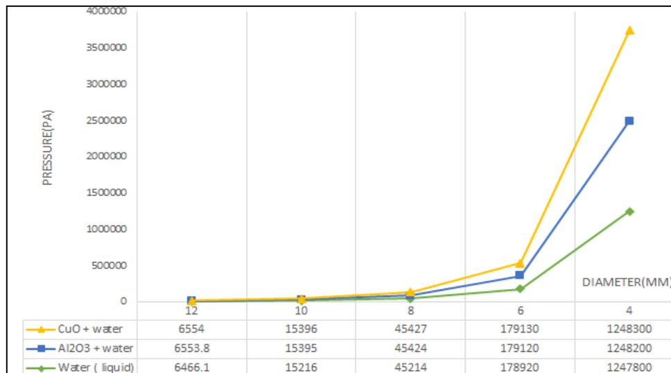
**Fig.3.1. Pressure versus diameters reading for Nano fluids**
