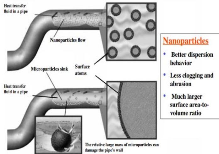
**Fig 1.1. Images of pipe analysis with and without Nano fluid particles**
