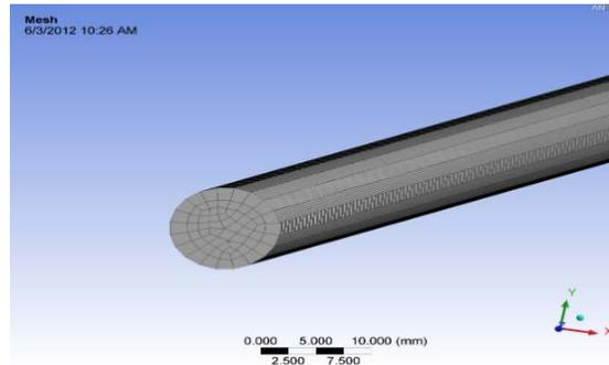
**Fig.2.2. Meshed Model of a circular pipe geometry**
