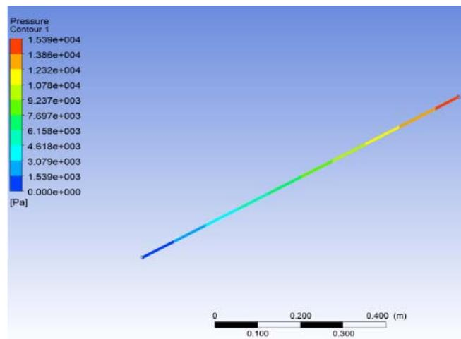
**Fig.2.5. Pressure counter diagram for Al<sub>2</sub>O<sub>3</sub> + water (liquid) particles**
