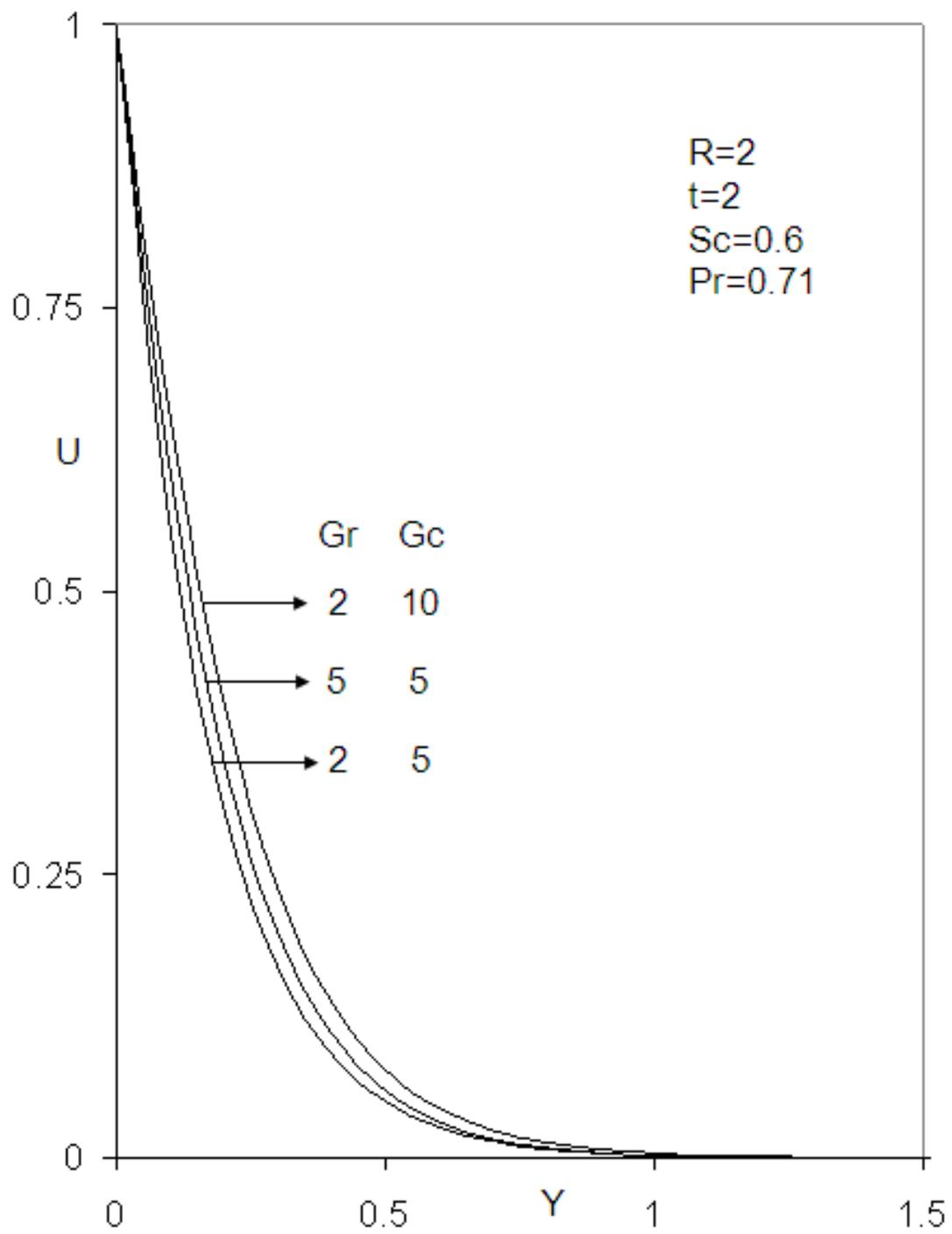
Fig.2. Velocity profiles for different Gr and Gc
