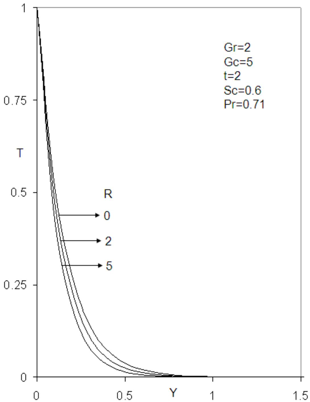
Fig.3. Temperature profiles for different R
