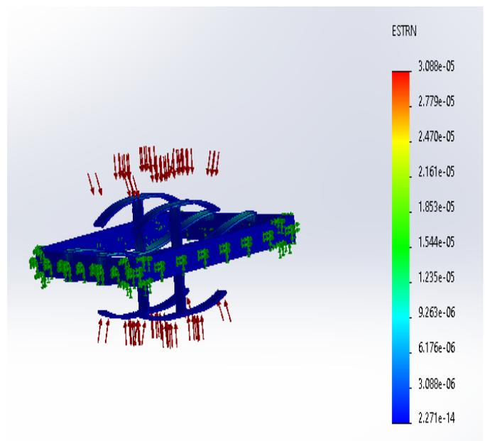
**Figure: 5** 1060 Aluminum alloy strain contour
