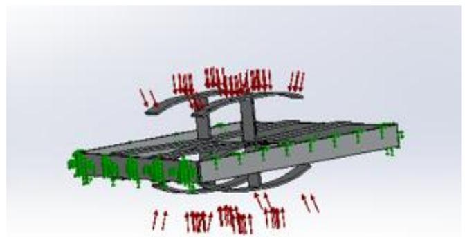
Figure: 2 Aircraft wing structure with boundary conditions
