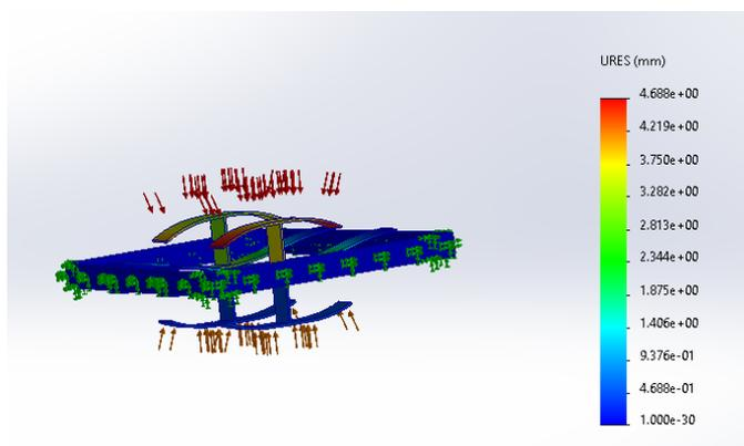
**Figure: 3** 1060 Aluminum alloy deformation contour
