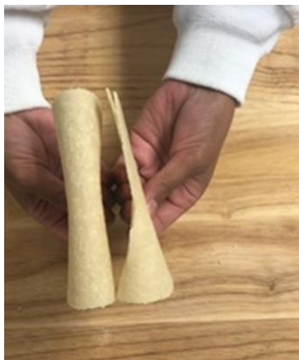
Fig. 3. Day 35 foldability for C9 (0.0100% high-performing maltogenic amylase) on the left and C1 (control) on the right
