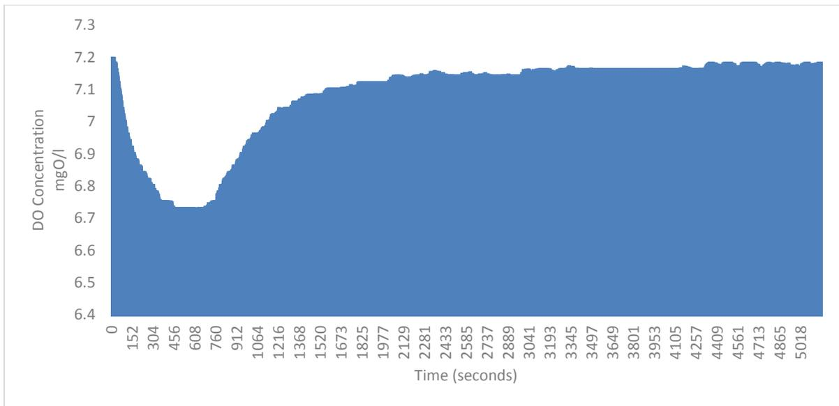
**Figure 7.** Dissolved oxygen response due to the addition of the 24hr filtered composite sample
