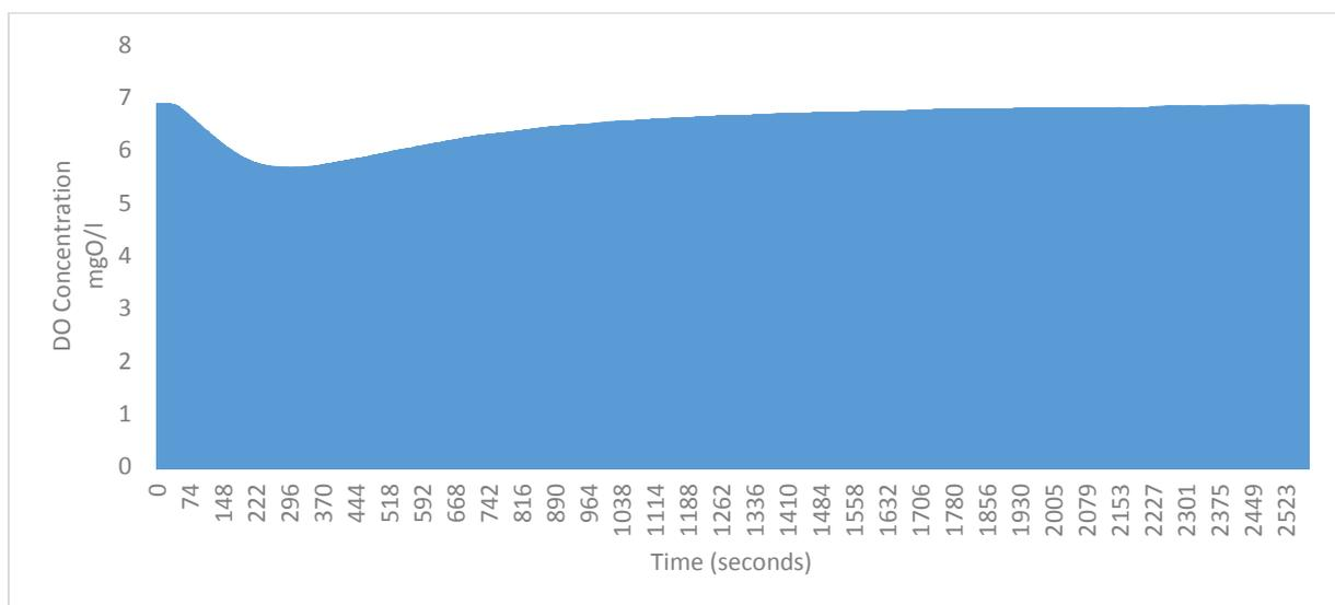
**Figure 5.** Dissolved oxygen response due to the addition of 24hr composite sample
