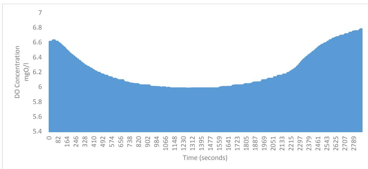
**Figure 3.** Dissolved oxygen response due to the addition of acetate
