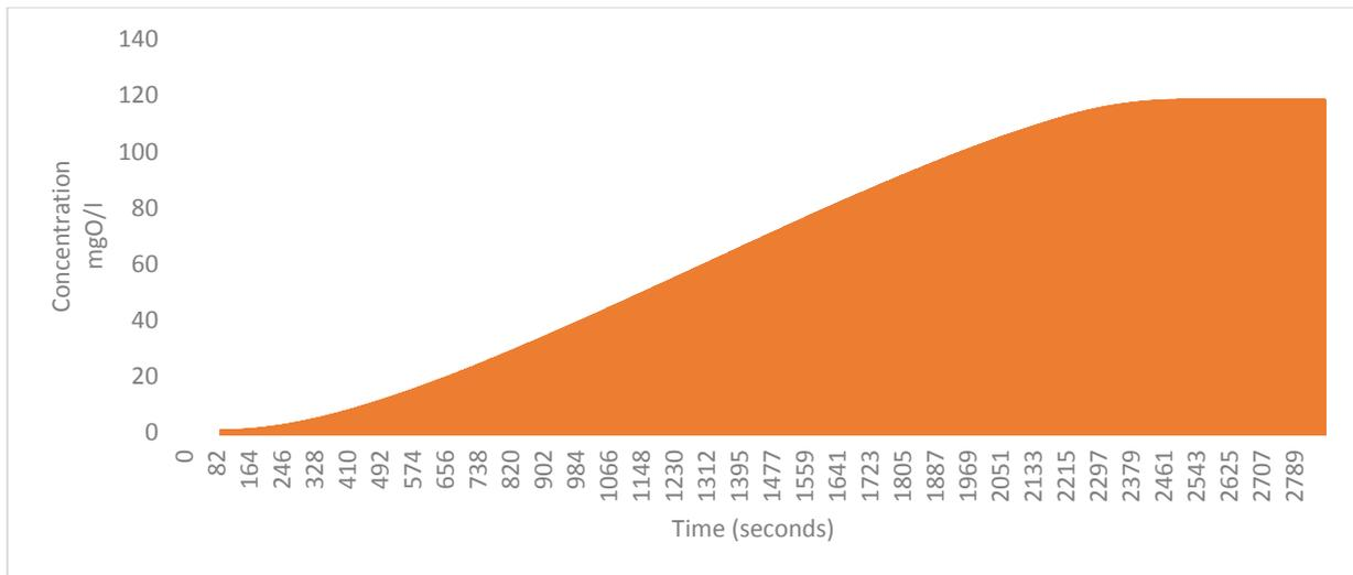
**Figure 4.** Consumed Oxygen response due to the addition of acetate
