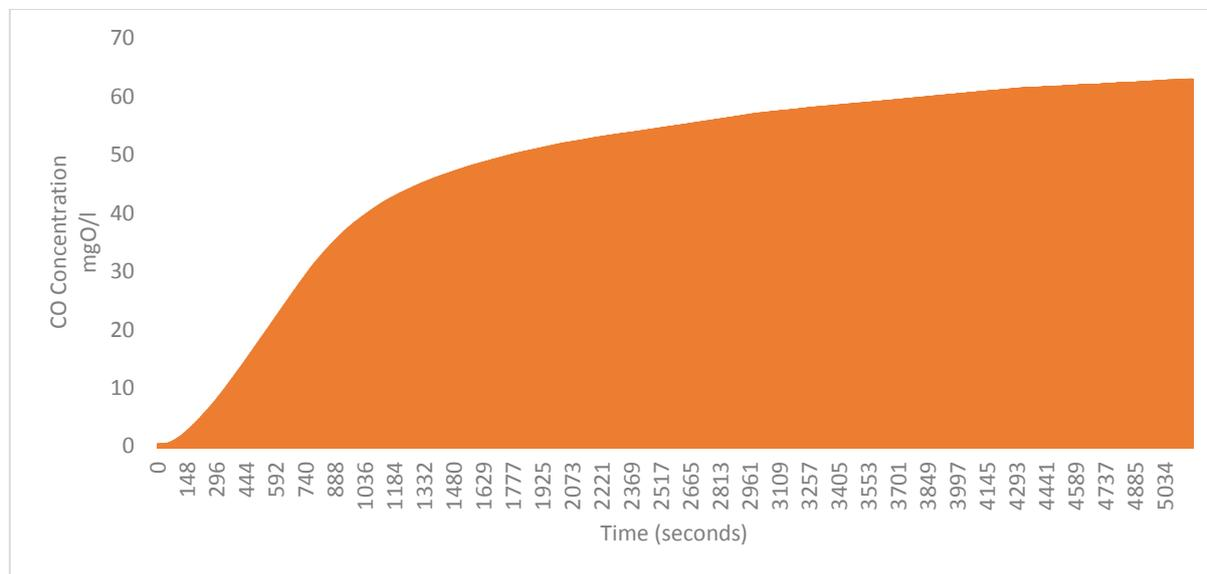
**Figure 8.** Consumed oxygen response due to the addition of 24hr filtered composite sample
