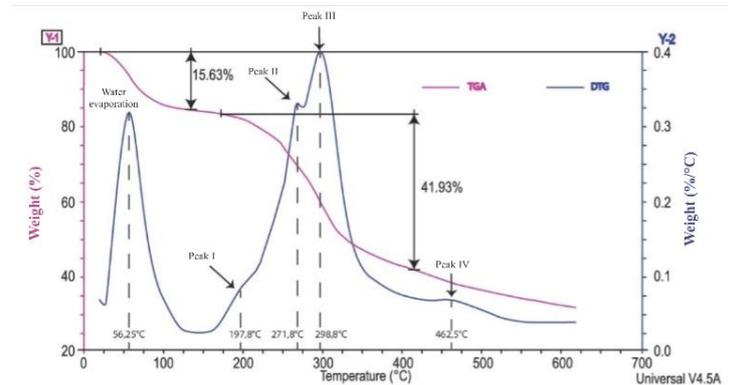
**Fig. 4.** CPH's TGA/DTG thermograms
