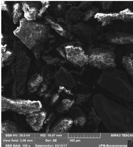
**Fig. 5.** Irregular amorphous structure of cocoa husk residues
