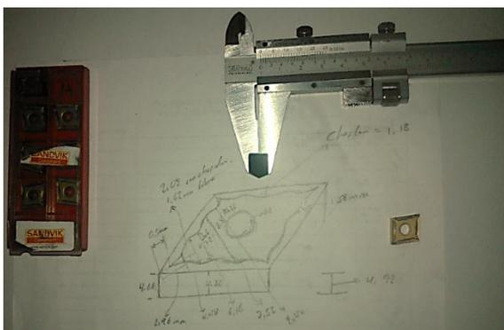
Fig. 56. Sketch of manual measurements of the insert.
