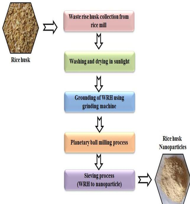
Fig. 2 Process involved in rice husk nano additive production
