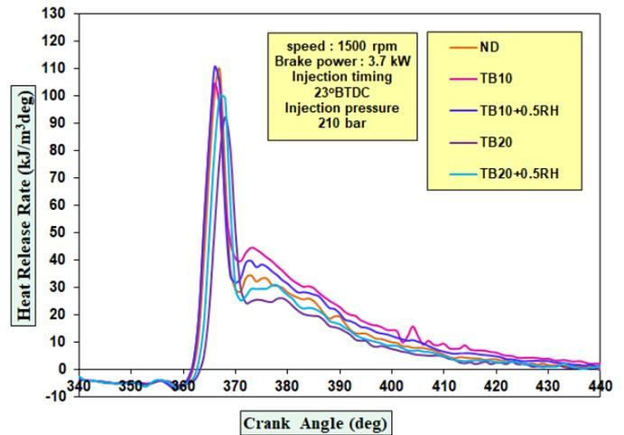
Fig. 11 Variation of HRR with crank angle
