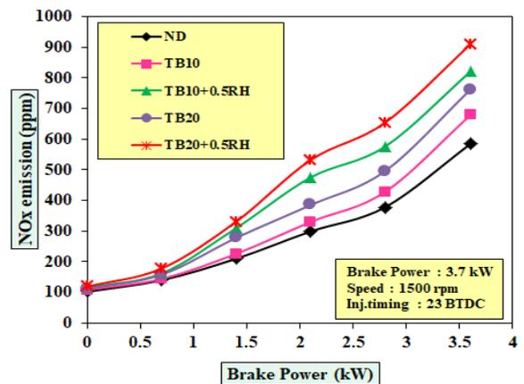
Fig. 7 Variation of NO<sub>x</sub> emission as a function of brake power
