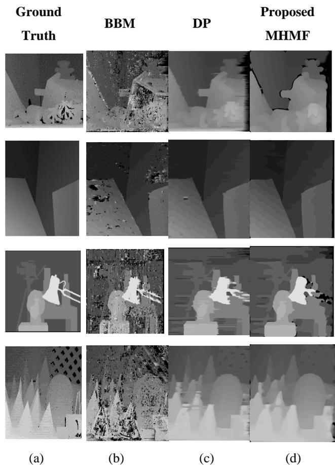
**Figure 8:** Results gained from the three stereo matching algorithms by applying the Middlebury benchmark datasets.
