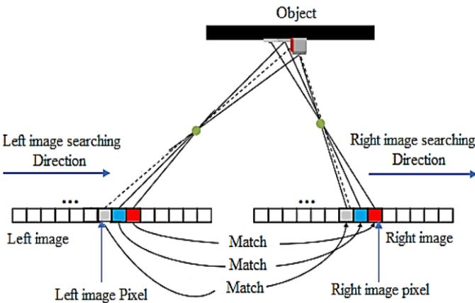
**Figure 4:** Example of the search of correspondence pixels between left and right stereo images
