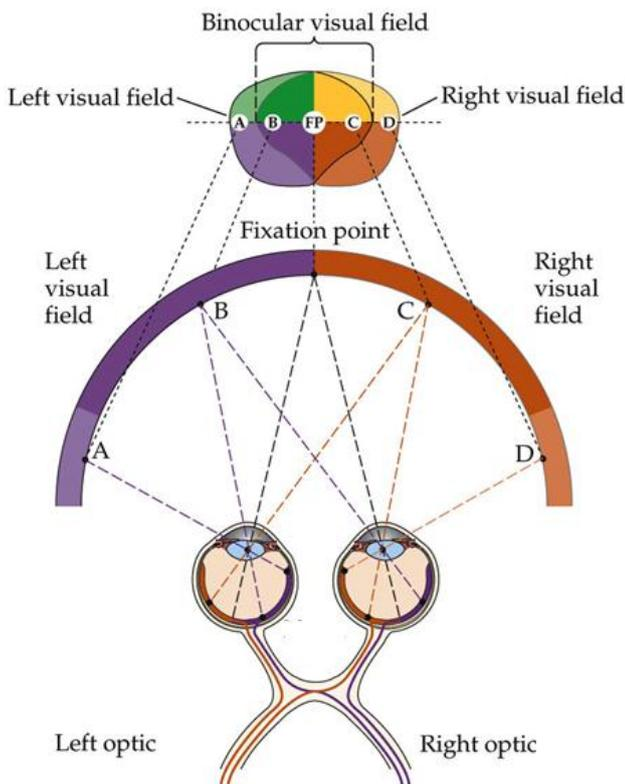
Figure 1. Human binocular vision processing principle [13]
