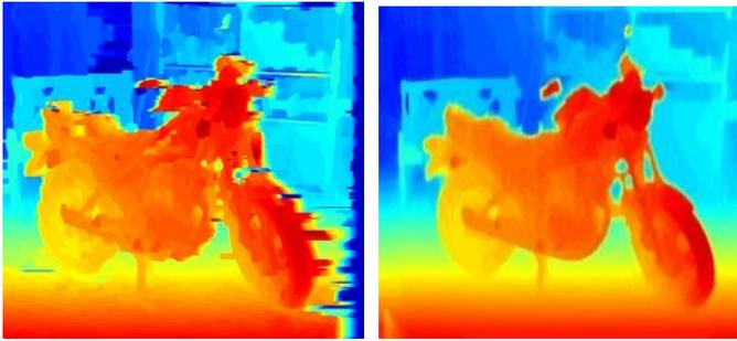
**Figure 6:** (b) Merge disparity map for Motorcycle image, (c) Final depth map for our proposed MHMF method.
