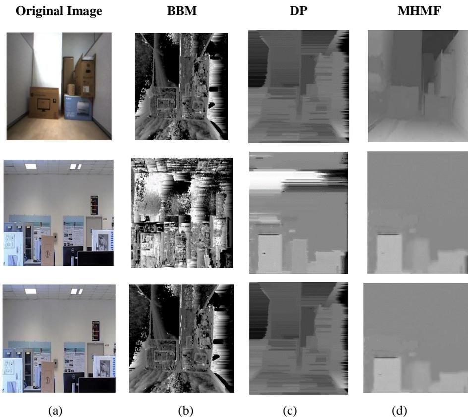
**Figure 7:** Results for stereo images captured with MV BLUEFOX camera: (a) Original stereo images; (b) Result from BBM; (c) Result from DP; (d) Result from MHMF.
