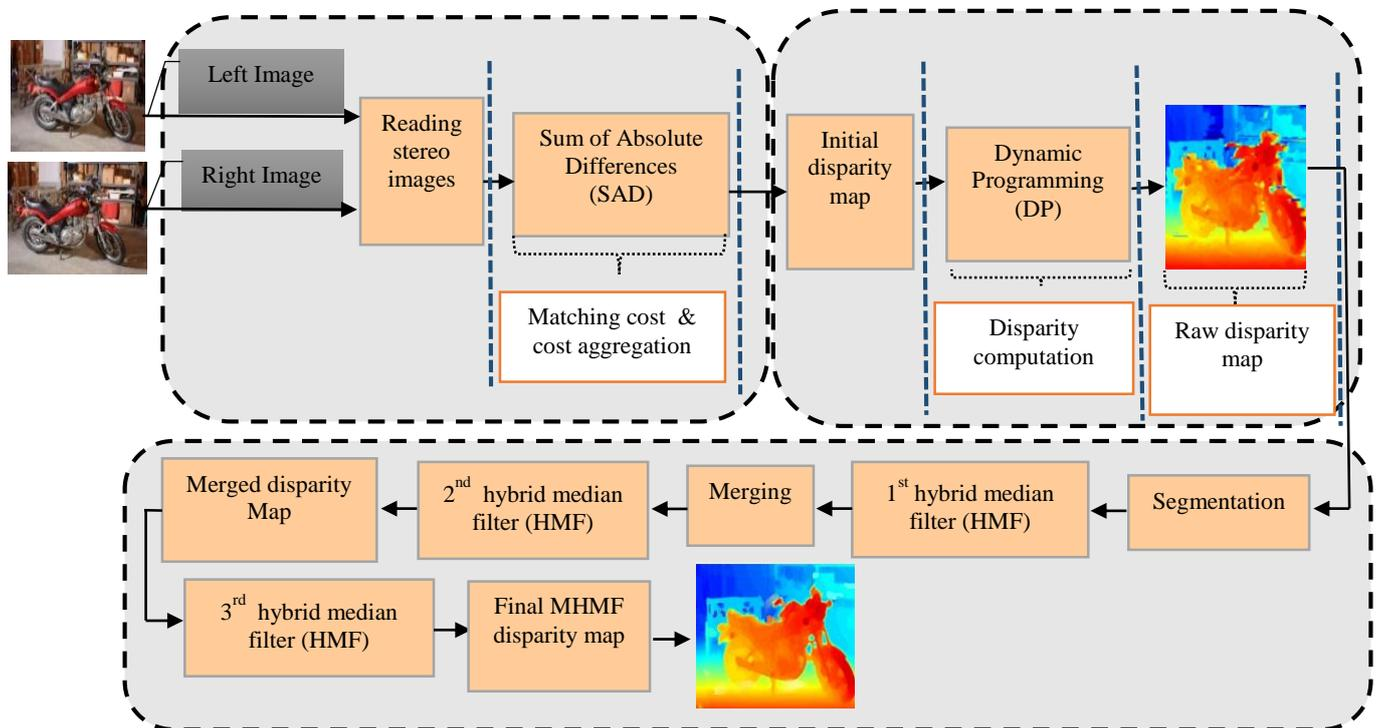
**Figure 3:** Overall structure of the proposed Multistage Hybrid Median Filter (MHMF) algorithm
