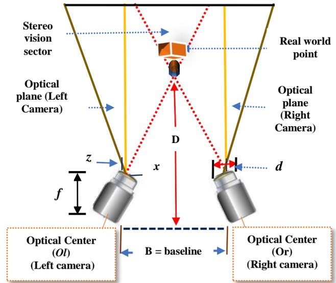
Figure 2: Binocular stereo vision (SV) principle basic structure
