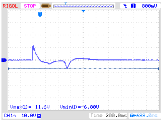
Fig. 4. One-step transducer electrical response using PLA
