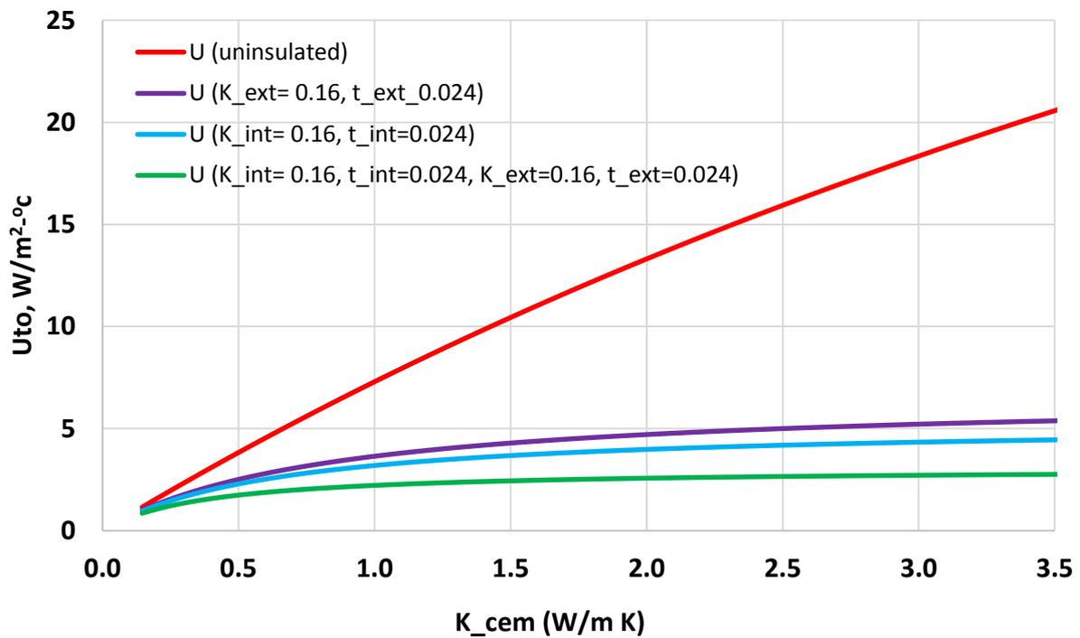
Figure 9: Overall heat transfer coefficient comparison between uninsulated and internal/external insulated tube
