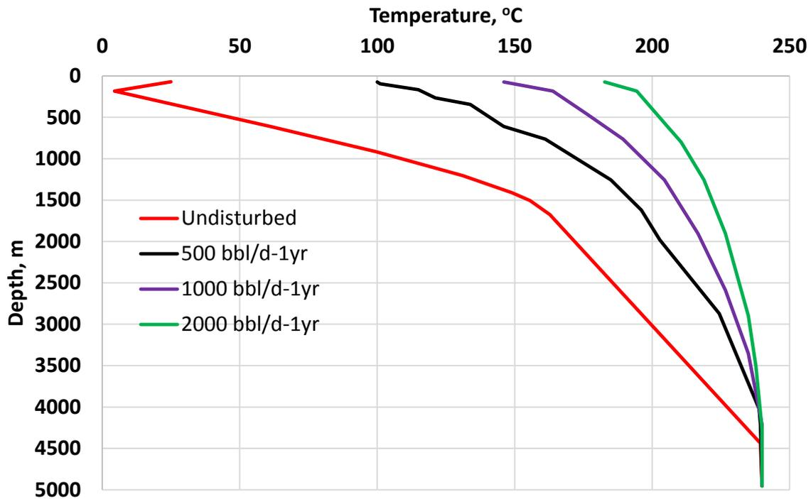
Figure 6: Tubing working fluid flowing temperature profile
