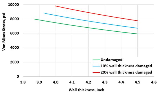
**Figure 2:** Stress analysis of undamaged and uniformly damaged tube
