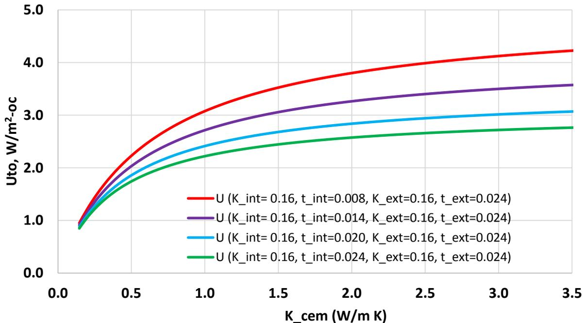
**Figure 11:** Effect of size of internal insulators on overall heat transfer coefficient.
