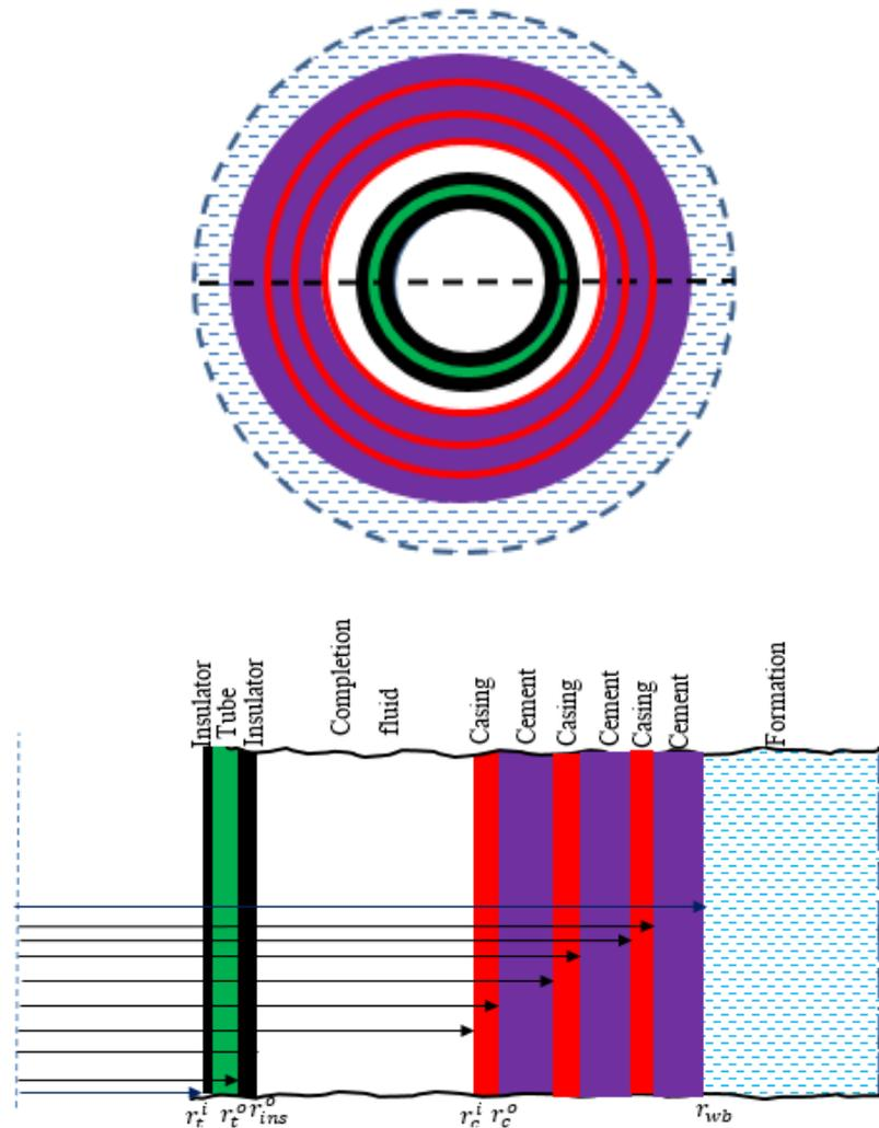
**Figure 8:** Illustration of the horizontal and vertical cross-section of the well
