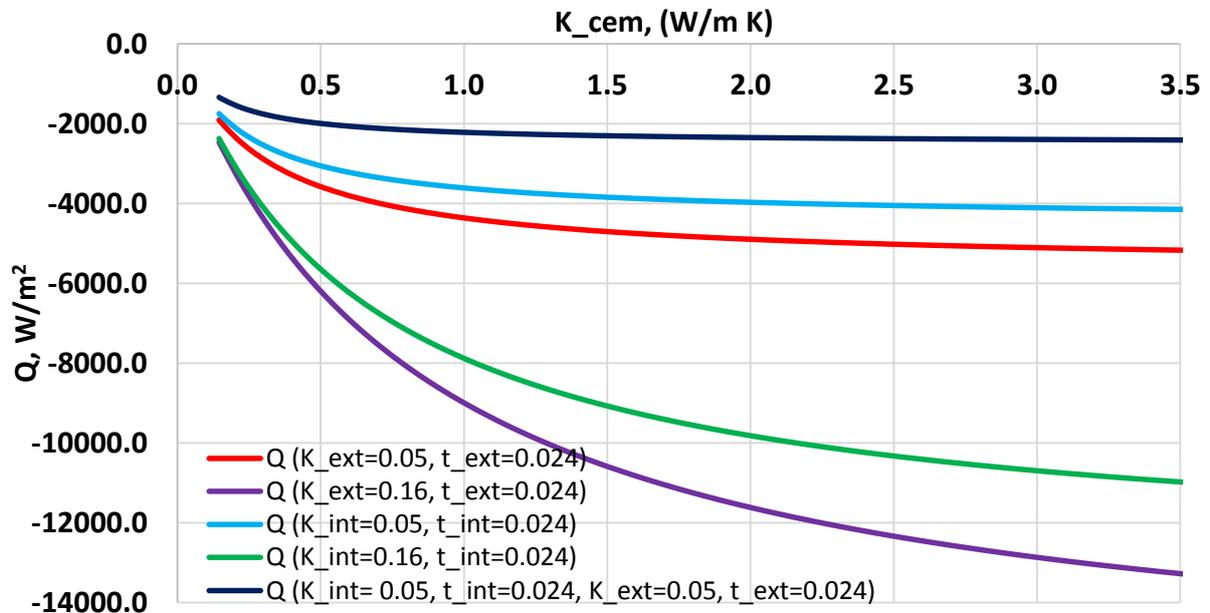
**Figure 14:** Effect of thermal conductivity and thickness of insulators on heat loss
