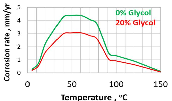
**Figure 4:** Effect of inhibitor on corrosion rate
