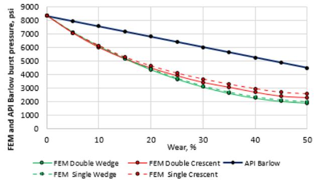
**Figure 3:** Comparison of tubing burst derated pressures of L-80 tube. (Belayneh et al., 2019)
