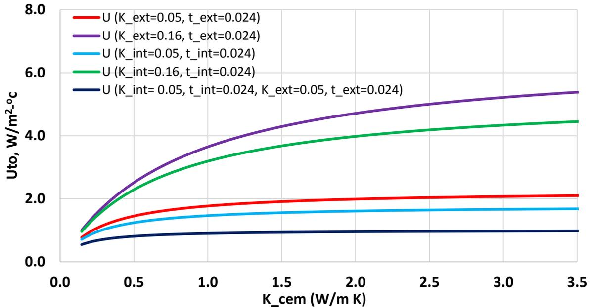
**Figure 13:** Effect of thermal conductivity and thickness of insulators on overall heat transfer coefficient.
