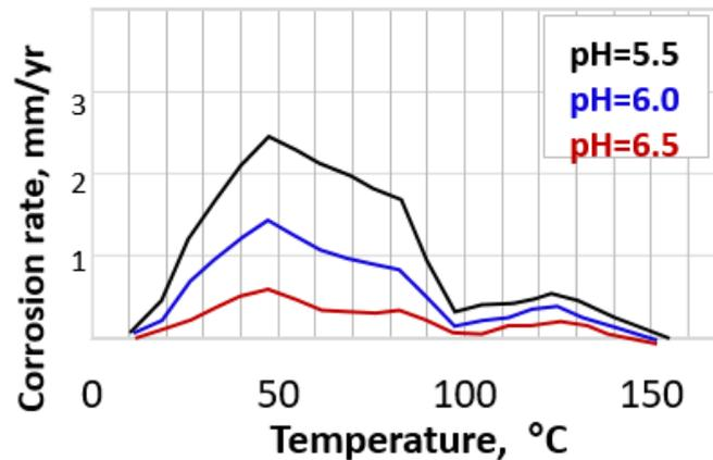
Figure 5: Effect of pH on corrosion rate
