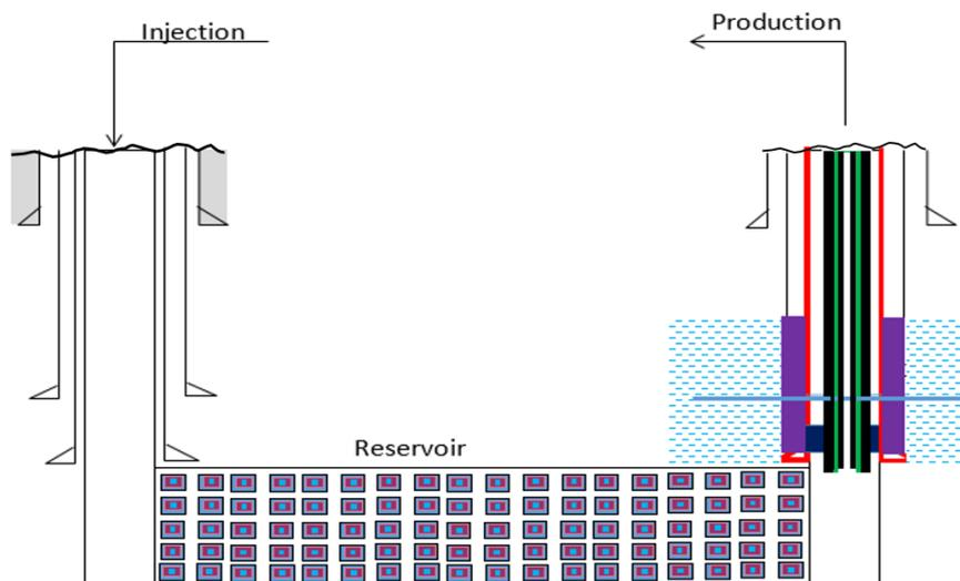
Figure 7: Illustration of geothermal injection/production and ideal dual porosity reservoir
