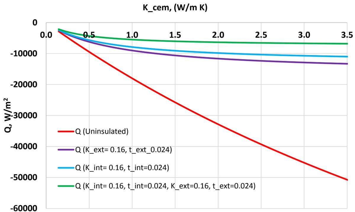
Figure 10: Heat loss comparison between uninsulated and internal/external insulated tube
