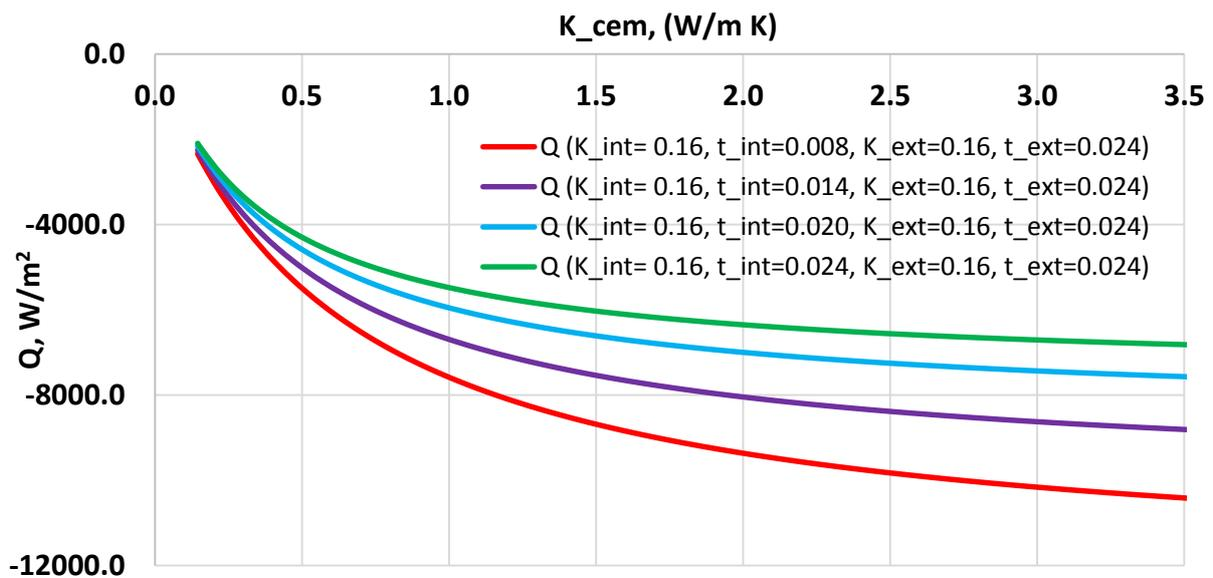
**Figure 12:** Effect of size of internal insulators on heat loss.
