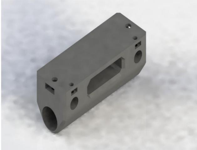
**Fig.4.** Design of part 4 (Y axis carriage) of the 3D printer.
