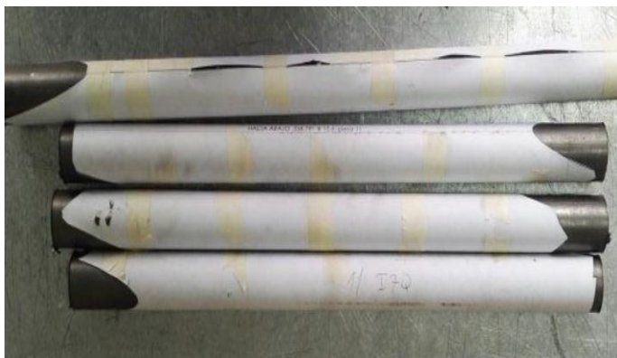
Fig. 2. Example of template guides for the cutting process of each structural member. Source: UPS Racing Team
