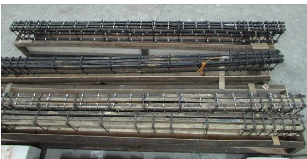
Fig. 3. The specimens of beam BRC of double reinforcement with hose-clamp and adhesive
