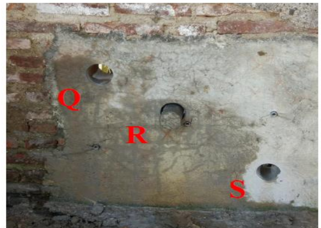
Fig 11. Core Drill sampling of retrofitted masonry wall
