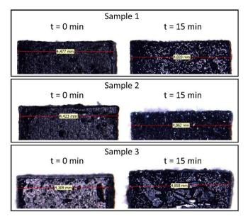
Figure 2 Swelling tests in electroplating electrolyte solution.
