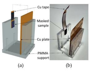
Figure 1 Electrodeposition setup: (a) CAD modeling and (b) actual setup.
