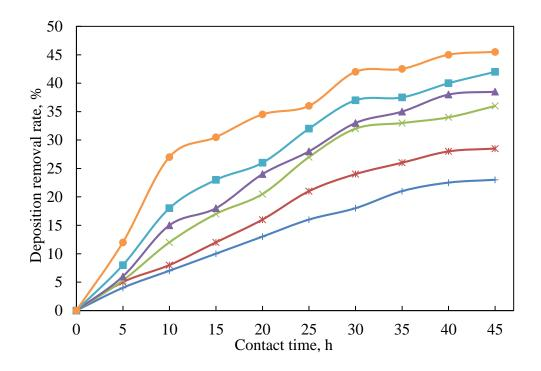
Figure 1. Kinetic curves of scale "washing off" at complexonate concentrations, where: -4 - 20 mg/kg; -4 - 15 mg/kg; -4 - 12 mg/kg; -8 mg/kg; -8 mg/kg; -4 mg/kg.
