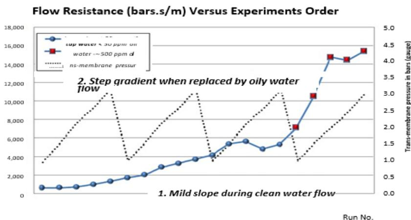
Figure 5: Decrease of flow resistance on the ceramic membrane 0.5  $\mu\text{m}$  was observed when trans-membrane pressure were gradually increased from 1.0 to 3.5 bar(g).
