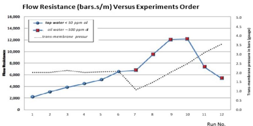
Figure 6: Increase of flow resistance on the 0.5  $\mu\text{m}$  pore size ceramic membrane due to fouling.
