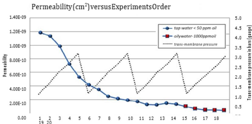
Figure 4: Permeability decline of ceramic membrane of 0.5  $\mu\text{m}$  pore size due to fouling.
