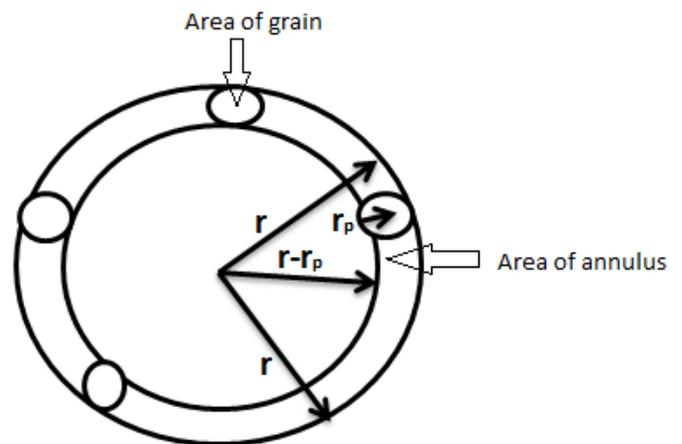
**Figure 1.** Schematic diagram of membrane channel showing grains, annulus and other parameters used to establish the expression for the maximum number of grains that can be coated in the membrane channel for proper wettability.
