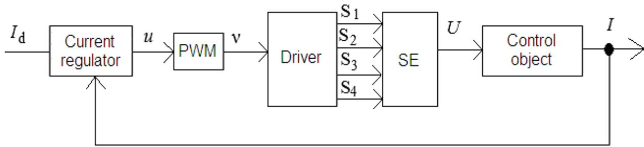
**Fig. 2.** Functional diagram of the control system for current flowing through the Peltier element
