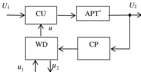
**Fig. 3.** Model of the amplitude-phase signal transformer with deviation control for analysis of TES
