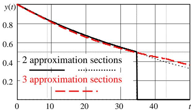
**Fig. 4.** Transients of the TEM ACS when approximating a nonlinear link with two or three linear sections
