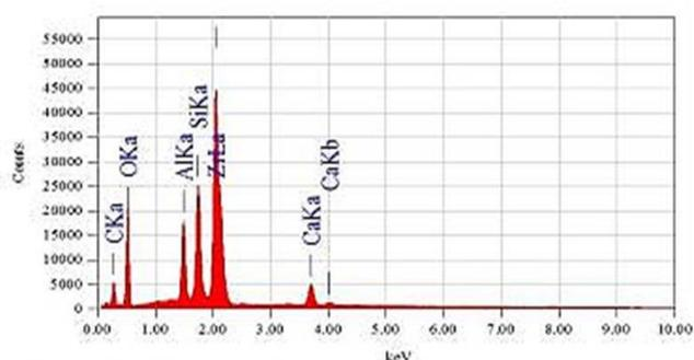
**Fig. 9** SEM-EDS qualitative analyses of CSZ pellet.
