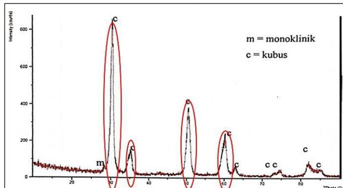
Fig. 6 XRD Standard Pattern of CSZ Pellet.
