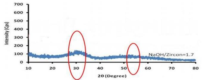
**Fig. 2** XRD standard pattern of  $Zr(OH)_4$  powder (indicated by red circle).
