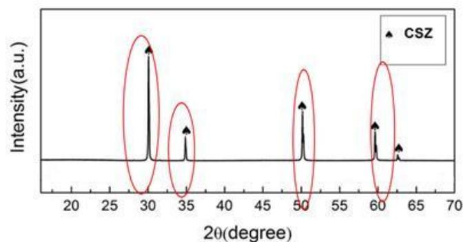
**Fig. 4** XRD standard pattern of CSZ powder.
