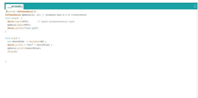
Figure 5. The code for Myoware Sensor and HC-06 Bluetooth Module
