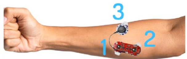
Figure 3. The way of connecting the myoware muscle sensor to the forearm muscles
