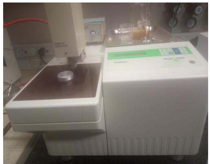
Figure 9. A Mettler Toledo (TGA/SDTA851) TGA Equipment (Department of Geology, University of Free State, South Africa)
