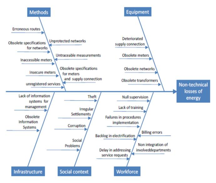
Figure 3: Causes of Non-Technical Losses in Distribution Systems
