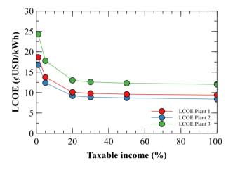
Fig 1b. Variation of the LCOE based on additional income.
