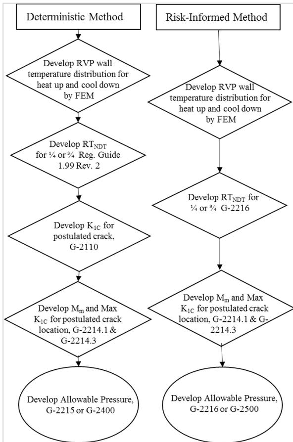
Figure 2: Procedure for constructing of P-T limit curves
