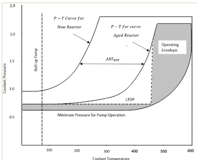
**Figure 1.** P-T operating envelop for RPV [5]
