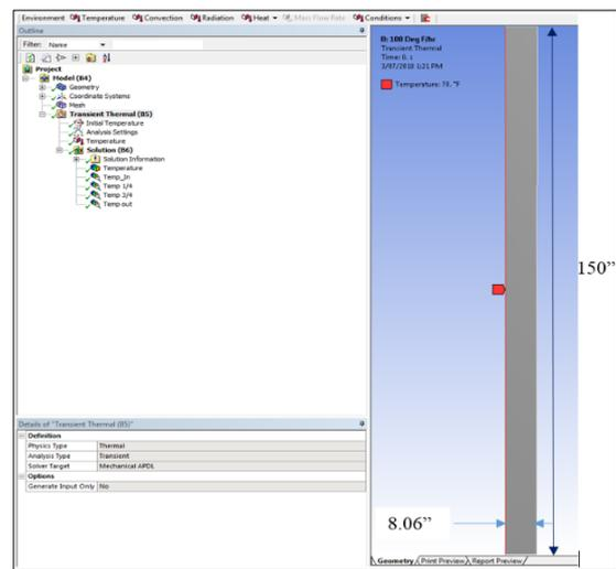
Figure 4. Thermal transient boundary conditions
