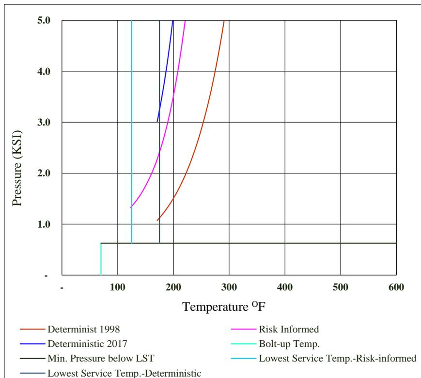
**Figure 7.** Comparison of P-T limit curves prior to 2006 Code with 2017 ed. – cooldown
