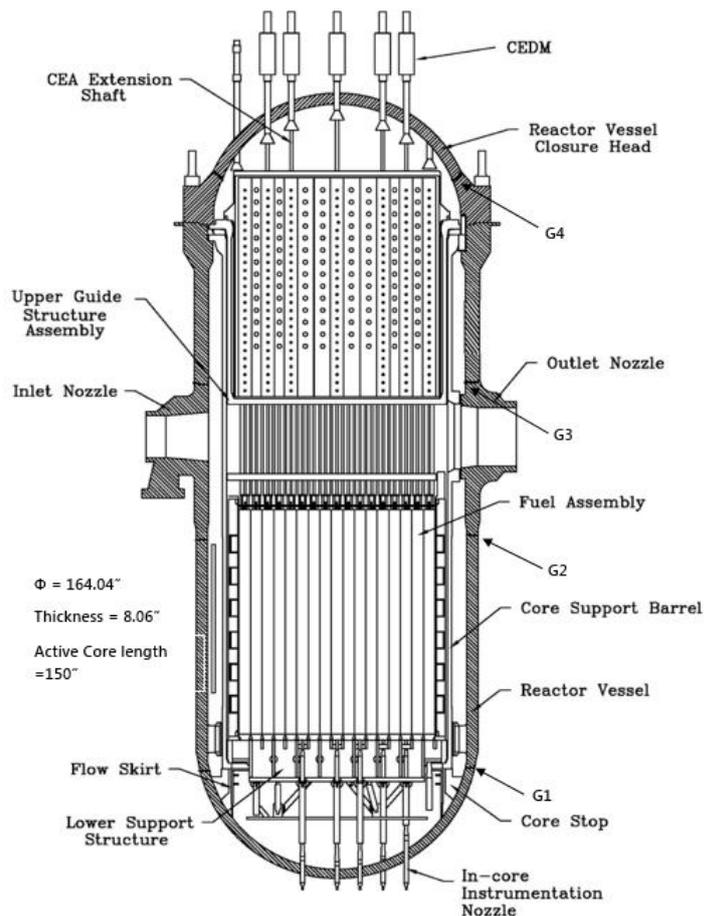
**Figure 2:** Nuclear Reactor Pressure Vessel Cross-section and Weld Regions Indicated by G-numbers [6]
