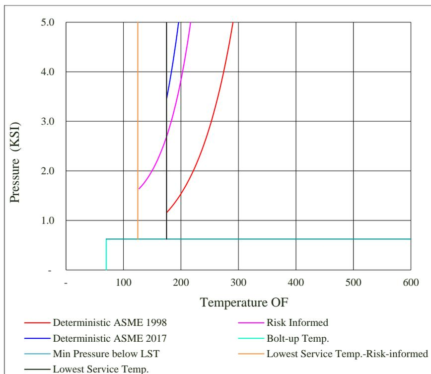
**Figure 8.** Comparison of P-T limit curves prior to 2006 Code with 2017 ed. – heat-up
