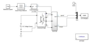
Figure 11. Implementation of NFSVPWM scheme in Simulink
