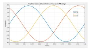
Figure 2. Balanced three phase ac voltage
