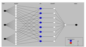
Figure 3. Neuro-Fuzzy network for position control of three phase induction motor
