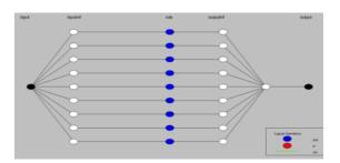
Figure 7. Neuro-fuzzy network for speed control of the three phase inductor motor
