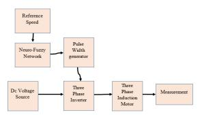
Figure 10. Integrated hybrid scheme for speed control of inductor motor
