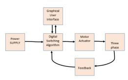
**Figure 1:** High level description of digital technique for Speed and Position of control three phase induction motor
