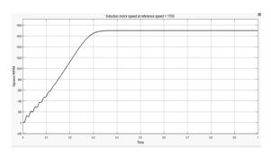
Figure 18. Response of NFSVPWM scheme at reference speed of 1700 rpm
