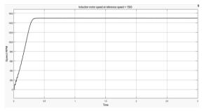
Figure 17. Response of NFSVPWM scheme at reference speed of 1500rpm
