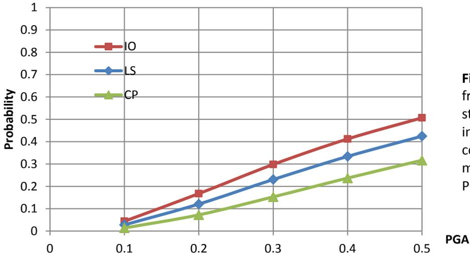
**Fig. 11** Seismic fragility of six stories fully infilled RC frame considering the medium class PGA/PGV ratio
