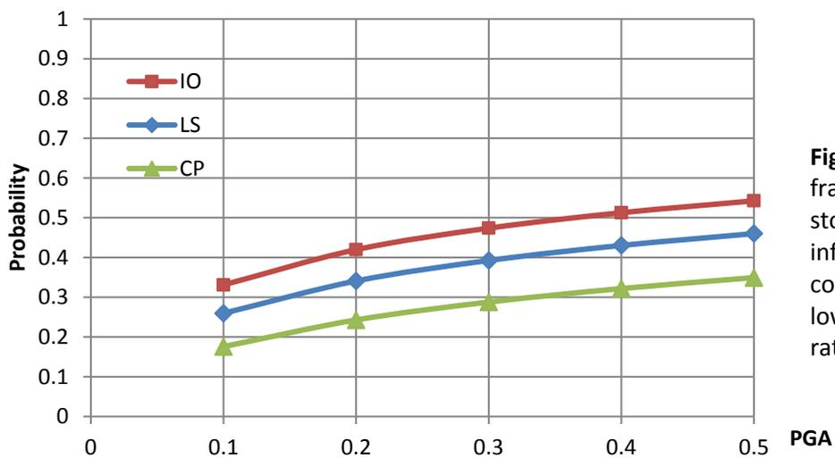
**Fig. 10** Seismic fragility of six stories fully infilled RC frame considering the low class PGA/PGV ratio
