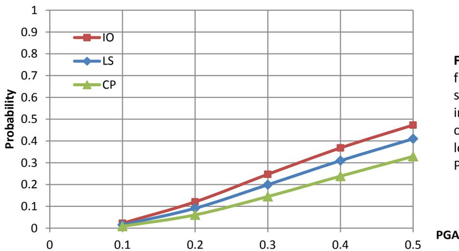
**Fig. 7** Seismic fragility of three stories fully infilled RC frame considering the low class PGA/PGV ratio
