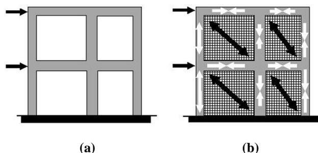
Fig. 1 Load transfer mechanism (a) bare frame (b) infilled masonry wall frame [1]
