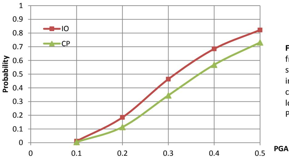
**Fig. 13** Seismic fragility of nine stories fully infilled RC frame considering the low class PGA/PGV ratio
