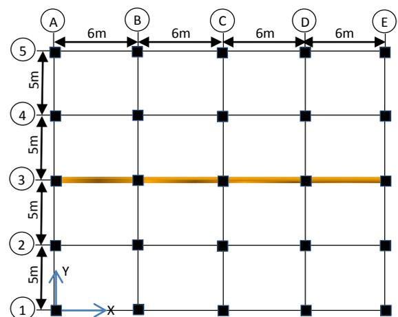
Fig. 2 Plan view of the building and the location of selected frame
