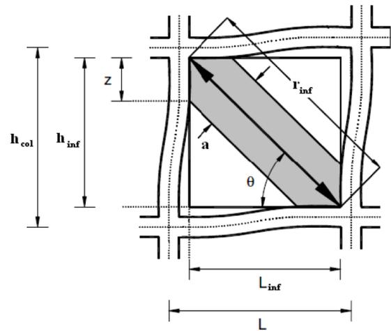
Fig. 4 Masonry infilled frame sub assemblages [23]
