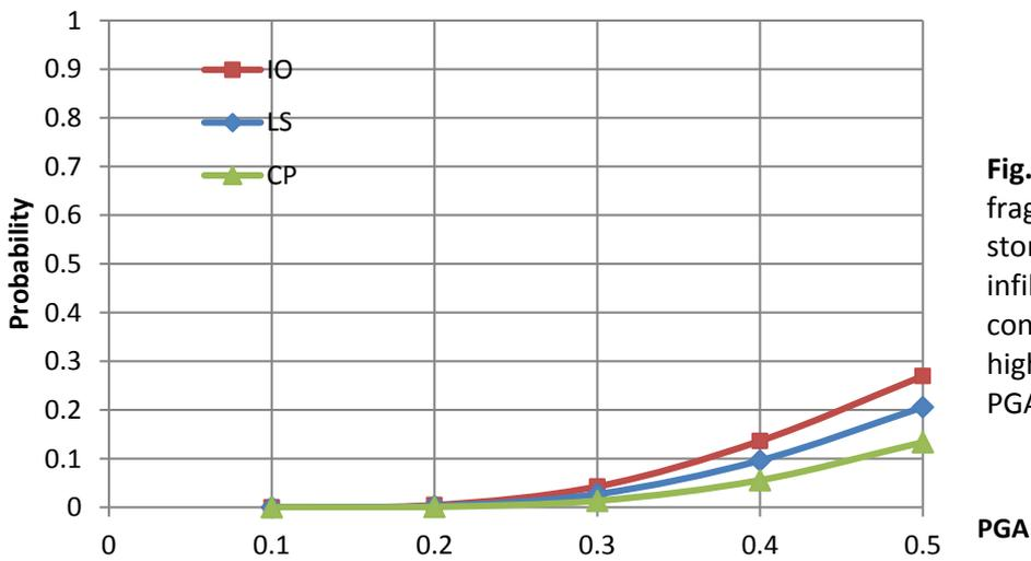
**Fig. 12** Seismic fragility of six stories fully infilled RC frame considering the high class PGA/PGV ratio
