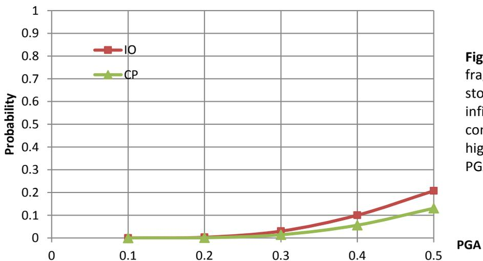
**Fig. 15** Seismic fragility of nine stories fully infilled RC frame considering the high class PGA/PGV ratio
