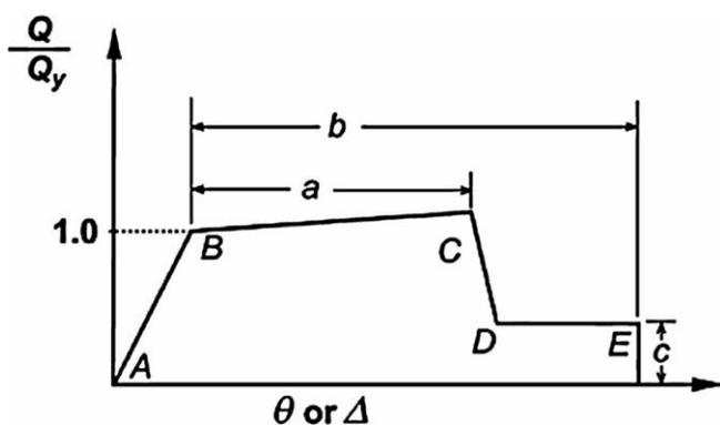
Fig. 3 Generalized chord rotation model used for inelastic behavior of beams and columns [19]
