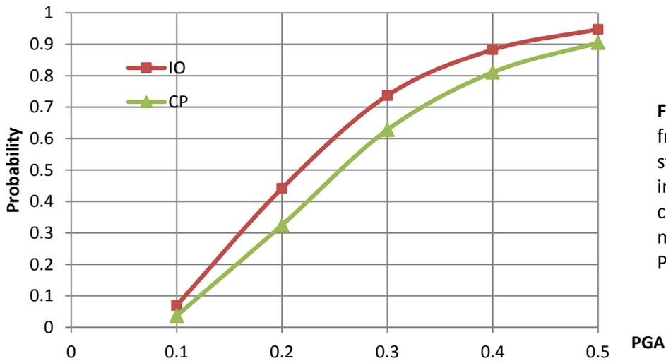
**Fig. 14** Seismic fragility of nine stories fully infilled RC frame considering the medium class PGA/PGV ratio
