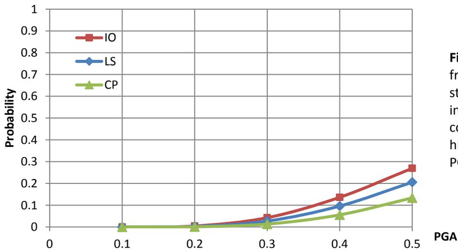
**Fig. 9** Seismic fragility of three stories fully infilled RC frame considering the high class PGA/PGV ratio
