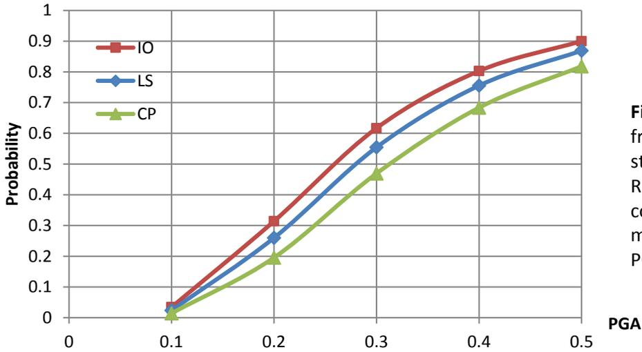
**Fig. 8** Seismic fragility of three stories fully infilled RC frame considering the medium class PGA/PGV ratio
