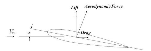
Figure 2. Aerodynamic forces [12, 14]
