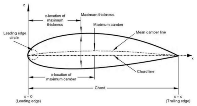
Figure 1. Airfoil-section geometry and it is nomenclature [11]
