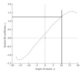
Figure 5. Lift coefficient vs. attack angle of NACA2412
