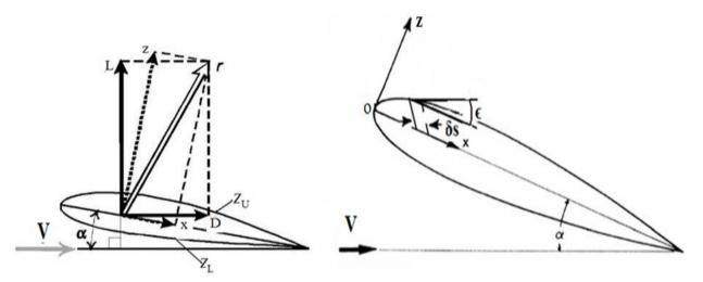
Figure 4. Normal pressure force on an element of the airfoil surface [15]
