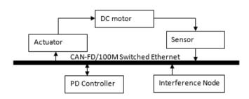
Fig. 2: A block diagram model of the NCSs. Fig. 2 illustrates how the different control components are interconnected through the network.
