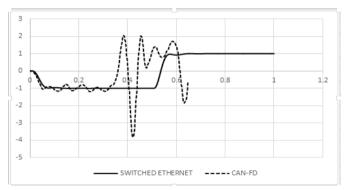
Fig. 12: Simulation results for each network when real-time network process is shared with other applications with an interference of 50%.
