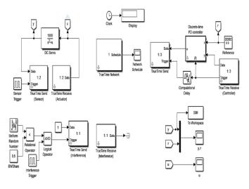
**Fig. 3:** NCS Model. Fig. 3 shows the NCS in-built model by Truetime kernel in the environment of Matlab/ Simulink 16b.
