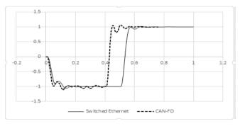
Fig. 6: CAN-FD and 100M Switched Ethernet networks with probability loss of 10%
