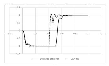
Fig. 9: CAN-FD and 100M Switched Ethernet networks with sampling period = 0.008 seconds
