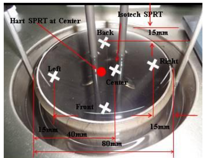
Fig. 4. Different positions of the Isotech SPRT for Horizontal and Vertical Uniformity Tests, excerpted from [8].
