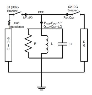
Figure 2: IEEE general system for islanding analysis
