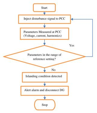
Figure 5: Flow chart of Active Method
