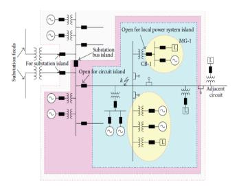
Figure 1: Illustration of Islanding Concept
