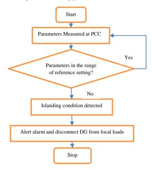
Figure 4: Flow chart for passive method
