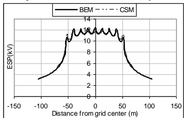
**Fig. C1:** Comparison between charge simulation method and Boundary Element Method for 64 meshes (75m\*75m) grid without vertical rods ( $\rho=2000 \Omega.m$ )
