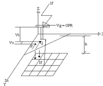
Fig. 3 Grounding system parameters, the ground potential rise (GPR), the fault current ( $I_f$ ), the touch voltage ( $V_t$ ), the step voltage ( $V_s$ ) and grid depth ( $h$ ) that computed to the proposed square grid [12]
