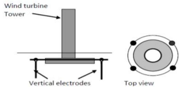
Fig. 1 Typical wind turbine grounding layout [10, 11]
