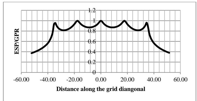
**Fig.8:** ESP/GPR for square grid buried on two layer soil
