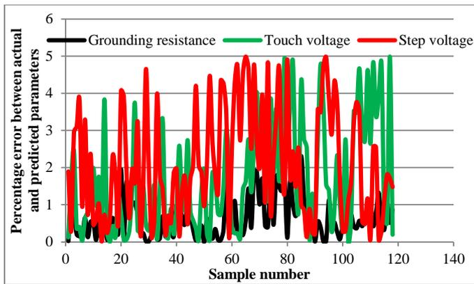
**Fig. 6:**Percentage error between the actual and predicted value of grounding resistance, touch and step voltages for two layer soil
