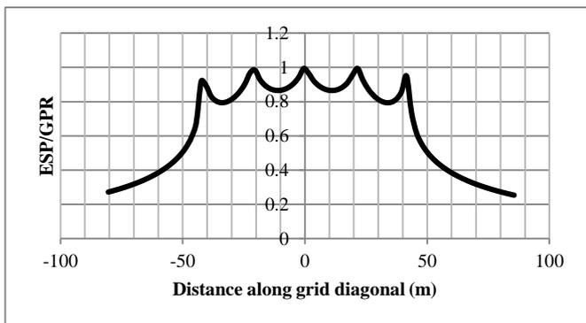
**Fig.7:** ESP/GPR for square grid in homogenous soil
