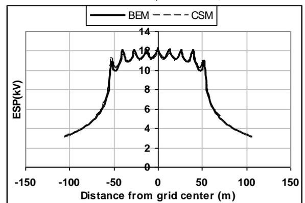
**Fig. C2:** Comparison between charge simulation method and Boundary Element Method for 64 meshes (75m\*75m) grid with vertical rods 2m and ( $\rho=2000 \Omega.m$ )
