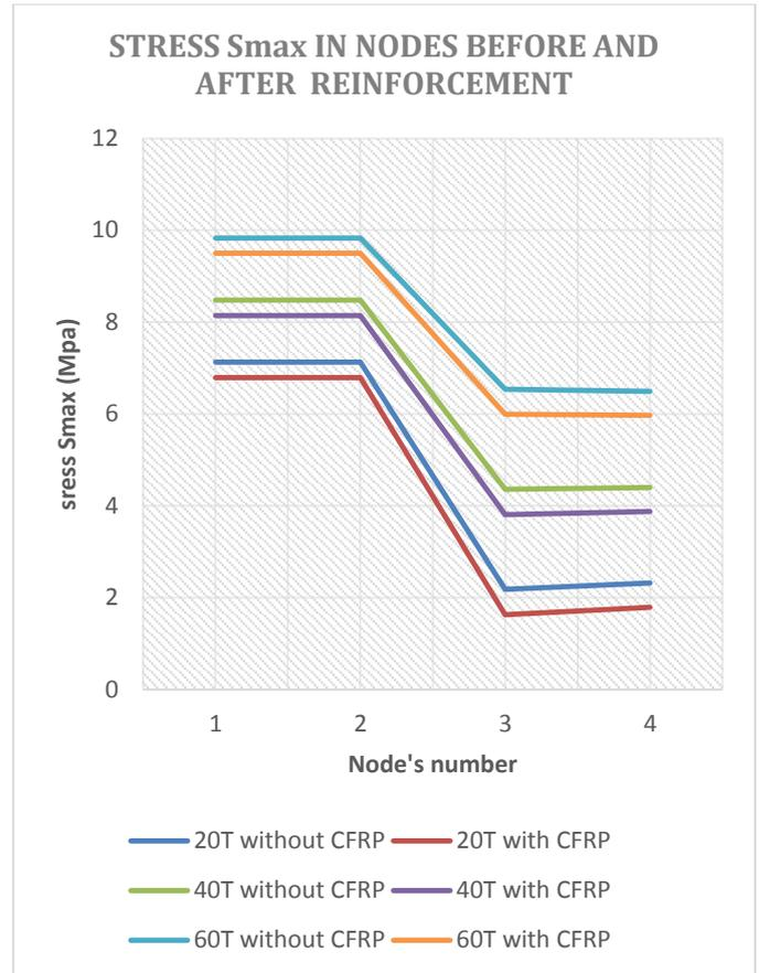
**Fig. 11.**  $S_{max}$  stress values in the node before and after reinforcement, depending on the loading applied 20,40 and 60T
