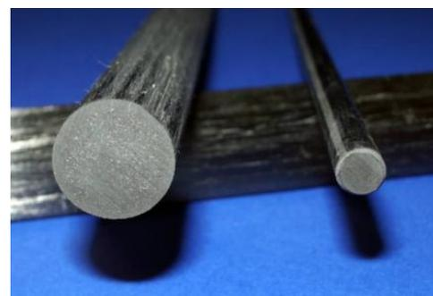
**Fig. 1.** Pultruded CFRP rods
