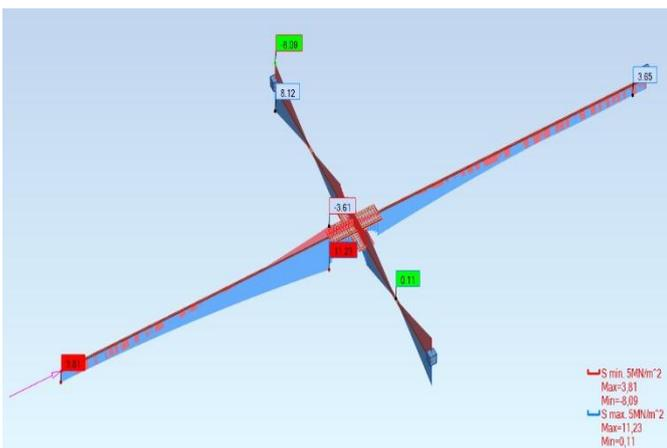
**Fig. 9.** Diagram of stresses in the bars with a reinforcement in CFRP for a horizontal effort of 40 T
