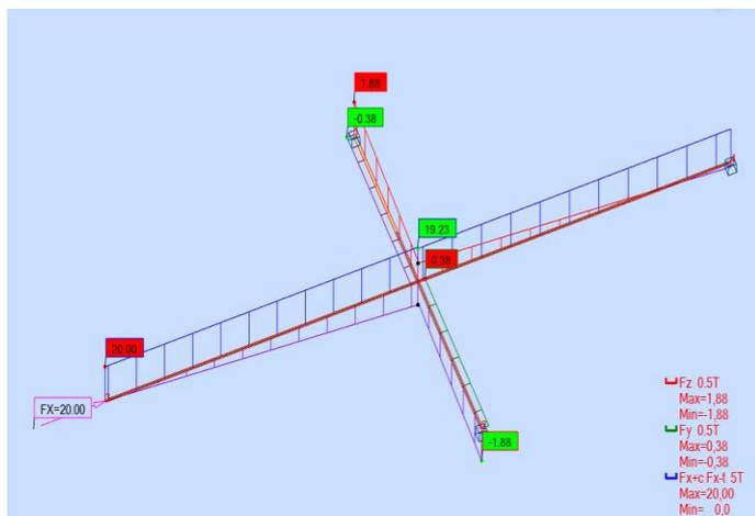
**Fig. 4.** Diagram of forces in bars without CFRP reinforcement
