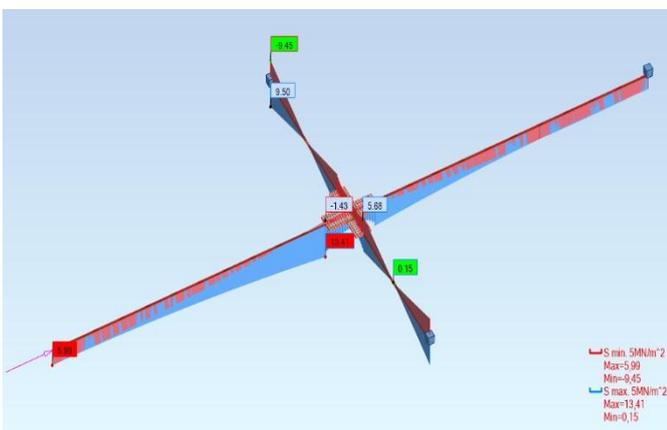
**Fig. 10.** Diagram of stresses in the bars with a reinforcement in CFRP for a horizontal effort of 60 T
