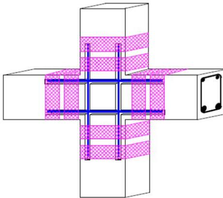
**Fig. 2.** The continuity of the reinforcement in a node ensured by CFRP rods
