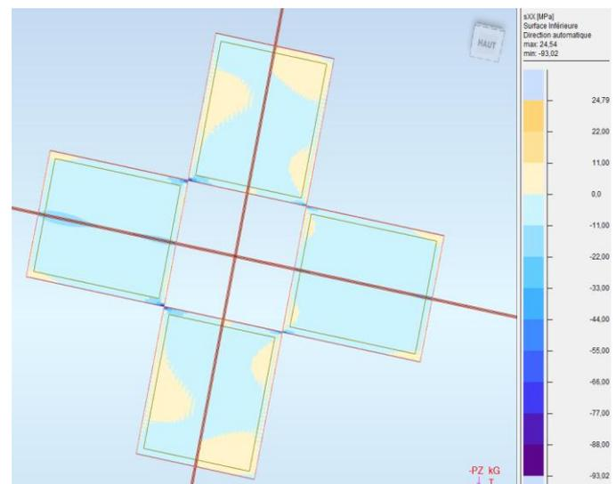
**Fig. 13.** Distribution of the Sxx stress in the CFRP tissue
