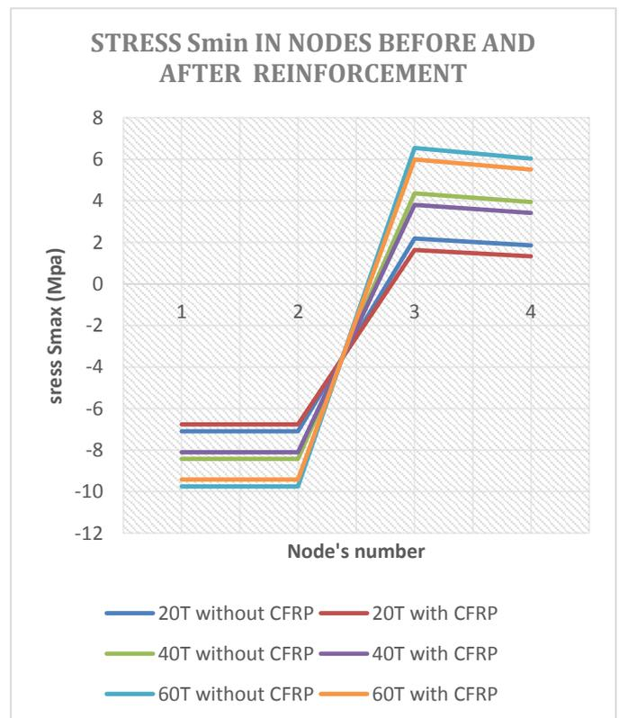
**Fig. 12.**  $S_{min}$  stress values in the node before and after reinforcement, depending on the loading applied 20,40 and 60T
