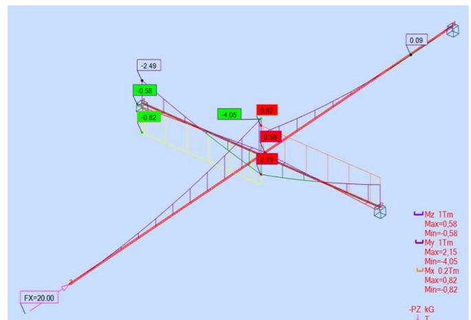
**Fig. 5.** Diagram of moments in bars without CFRP reinforcement
