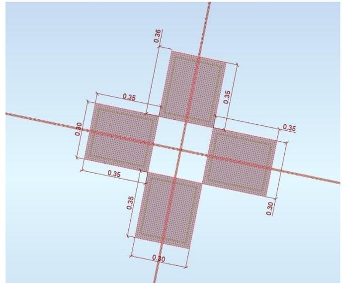
**Fig. 7.** The junction of CFRP panels (30x35 cm<sup>2</sup>) with column and beam constituting the Node
