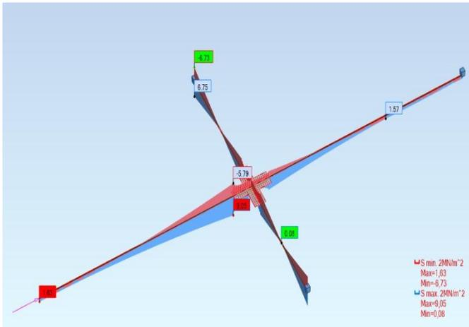
**Fig. 8.** Diagram of stresses in the bars with a reinforcement in CFRP for a horizontal effort of 20 T
