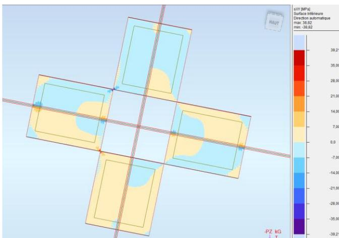
Fig. 15. Distribution of the Sxy stress in the CFRP tissue
