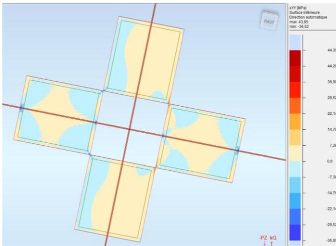
Fig. 14. Distribution of the Syy stress in the CFRP tissue
