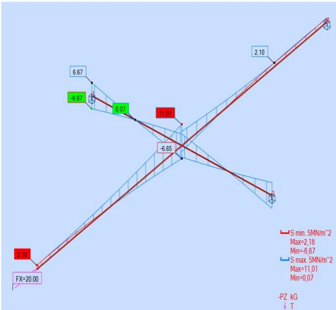
**Fig. 6.** Diagram of stresses in bars without CFRP reinforcement
