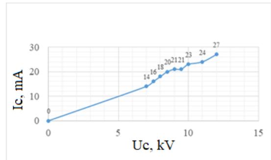
Fig. 8. Current-voltage characteristic of the ozonizer.
