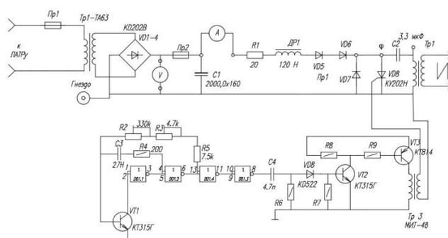
Fig. 7. Thyristor high-voltage inverter with a master oscillator
