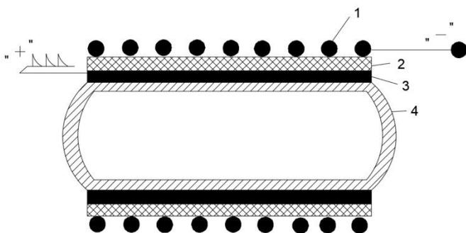
Fig. 5. Design of an ozonizing element on a corona-barrier discharge: 1 - corona electrode-microwire; 2 - a barrier of a dielectric material-fluoroplastic; 3 - the second electrode is a metal foil; 4 - a cylindrical flask from a dielectric - glass, ceramics.
