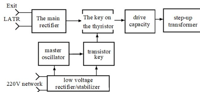
Fig. 6. The structural diagram of THVI
