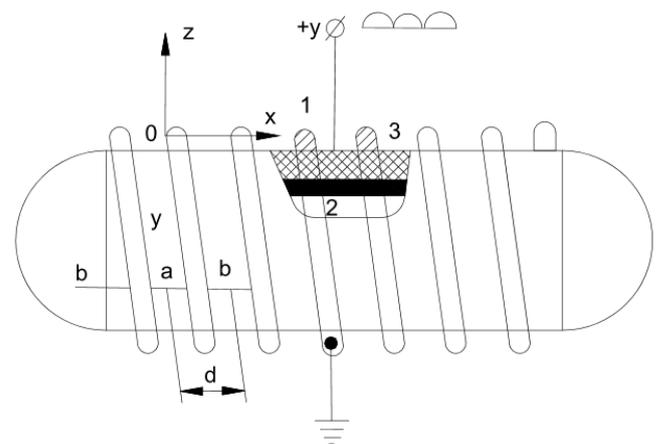
**Fig. 2.** The design scheme of the ozonizing element: 1 - spiral, 2 - second electrode, 3 - glass cylinder
