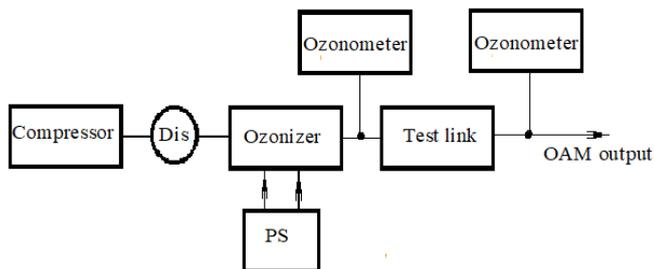
Fig. 4. The structure diagram of the experimental setup
