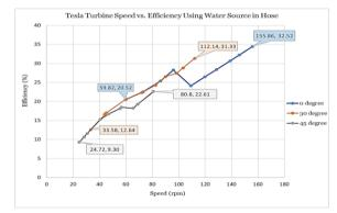
Figure 3.5. Efficiency and Speed relationship in a hose water flow
