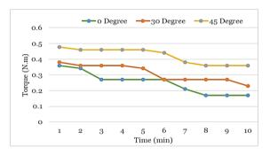
Figure 3.8. Torque and time relationship in a weir water flow
