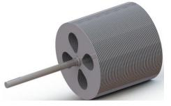
Figure 1.2. Number of angular discs of Tesla turbine mounted on the shafting
