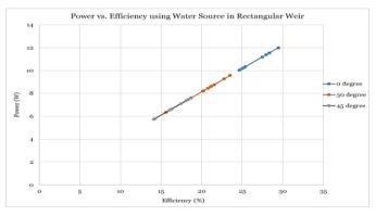
Figure 3.11. Power and efficiency relationship in a weir water flow
