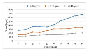
Figure 3.7. Speed and time relationship in a weir water flow
