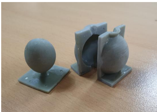
Fig. 8. Mold manufactured using 3D printed artificial testicle
