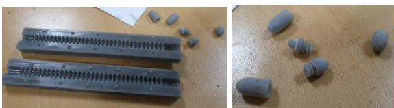
Fig 6. Printed Mold and Model (Left) / Post-Processed Model (Right)
