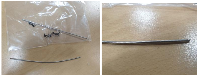
Fig 4. SUS304 Wire (Left) and Wire in Spring Form (Right)
