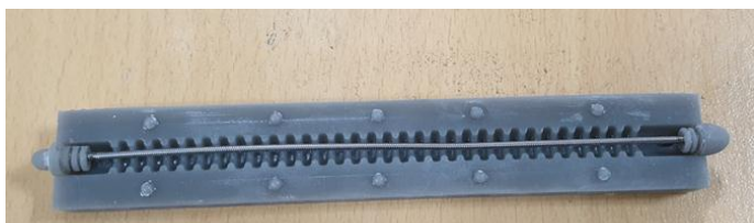
Fig 7. Rotation Axis Fixed in the Mold for Reproduction
