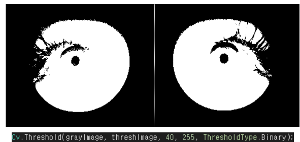
Fig. 4. Source code for converting the image to black and white
