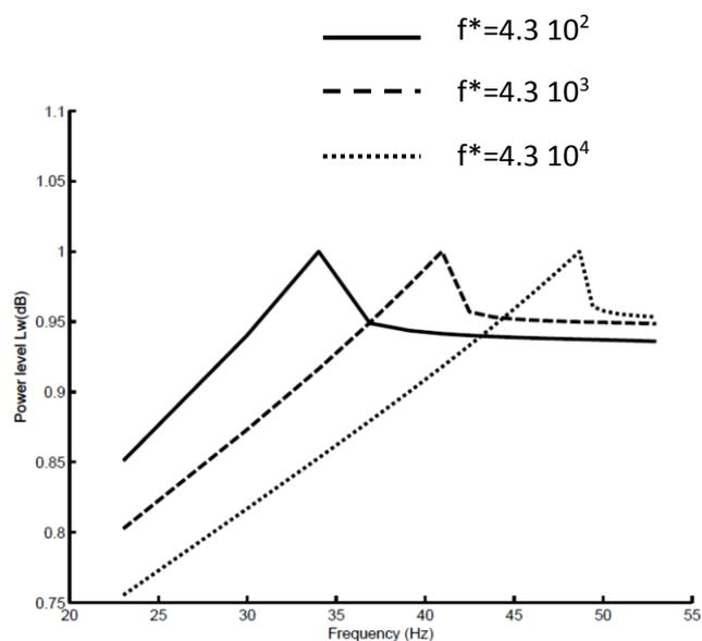
**Fig.7.** Normalized nonlinear power level in the neighborhood of the first mode for different values of the dimensionless excitation force
