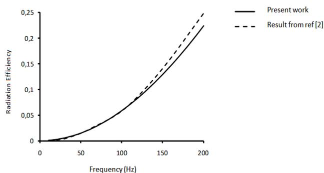
Fig.3. Radiation Efficiency of a simply supported plate
