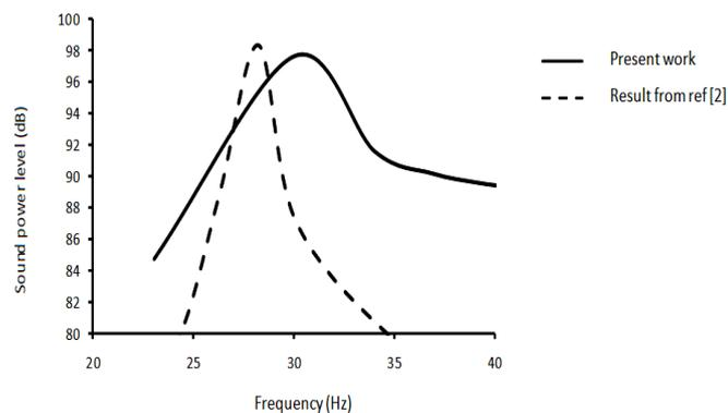
**Fig.4.** Linear sound power level radiated from a simply supported plate
