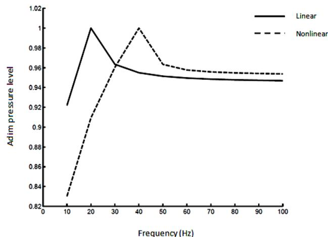
**Fig.6.** Normalized linear and nonlinear pressure level in the neighborhood of the first mode for  $f^*=1434$ .
