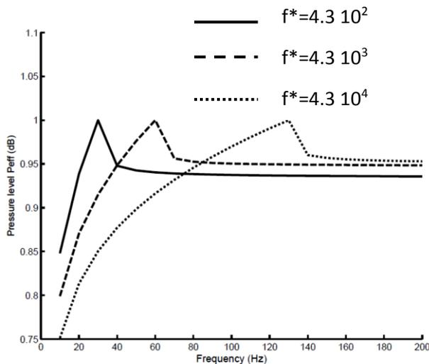
**Fig. 8.** Normalized nonlinear pressure level in the neighborhood of the first mode for different values of the dimensionless excitation force
