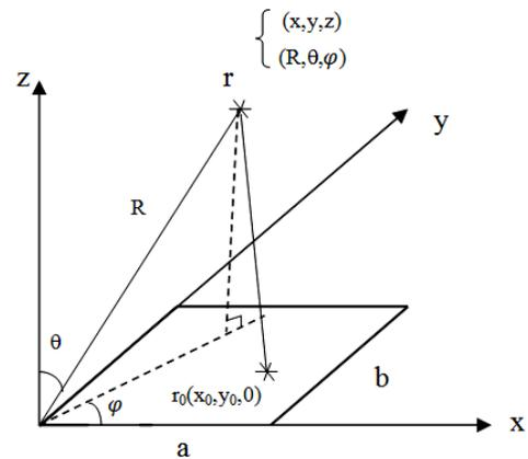
Fig.1. A rectangular thin plate in flexural vibration and its co-ordinates
