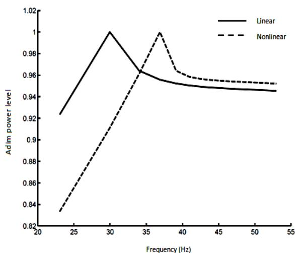
**Fig.5.** Normalized linear and nonlinear power level in the neighborhood of the first mode for  $f^*=1434$
